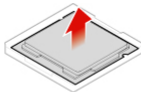
Figure 116. Pivoting the microprocessor socket upward
