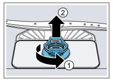
Pull down the micro filter to remove.
