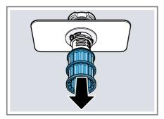
4. Press the locking catches 1 together and lift the coarse filter out
