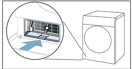
**10.** Slide the heat exchanger cover in by its grip.
