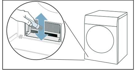
**Note:** Always clean the fins on the heat exchanger from top to bottom, taking care not to bend or damage them.
