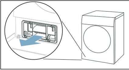
5. Carefully remove the filter mat from the heat exchanger cover.
