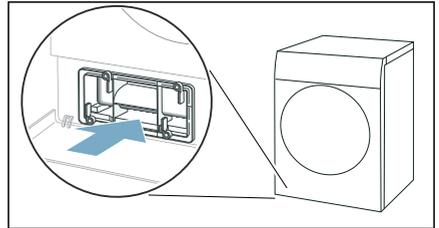
**Note:** You can only slide the heat exchanger cover in if the insert is in the appliance.
