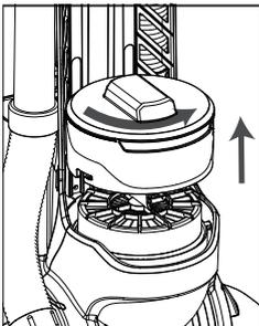
2. Remove the post motor filter by lifting it.
