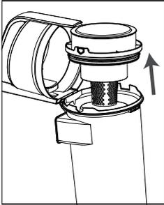
3. Remove the motor and sponge filter from the separator.
