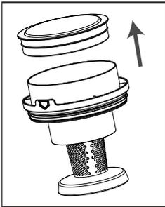
4. Wash the pre-motor filter with warm water until it gets clean (let the clean filter to dry 24 hours).
