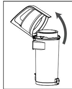
2. Hold and turn the separator clockwise from its handles and take it out from the dust container.
