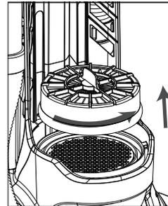
3. Wash the post motor filter with warm water until it gets clean (let the clean filter to dry 24 hours).
