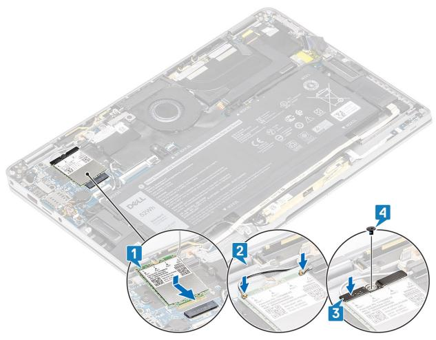
5. Place the metal shield on the WWAN card.
