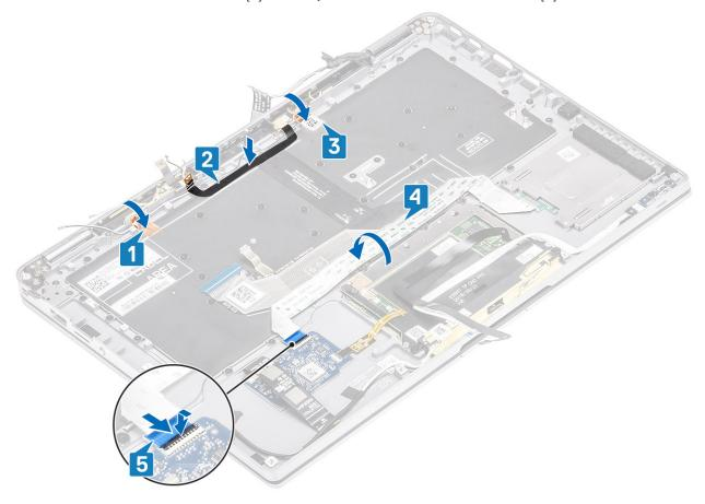
8. Stick the USH board cable [1], touchpad cable [2], and LED board cable [3] on the keyboard base.
