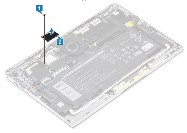
**4.** Slide and remove the SSD module from the connector on the system board.
