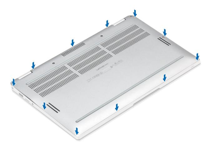
${\bf 3.}\ \ \, {\rm Tighten}$  the 10 captive screws to secure the base cover to the computer.
