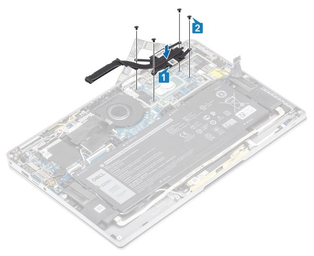
**3.** Place the heatsink shield on the heatsink.
