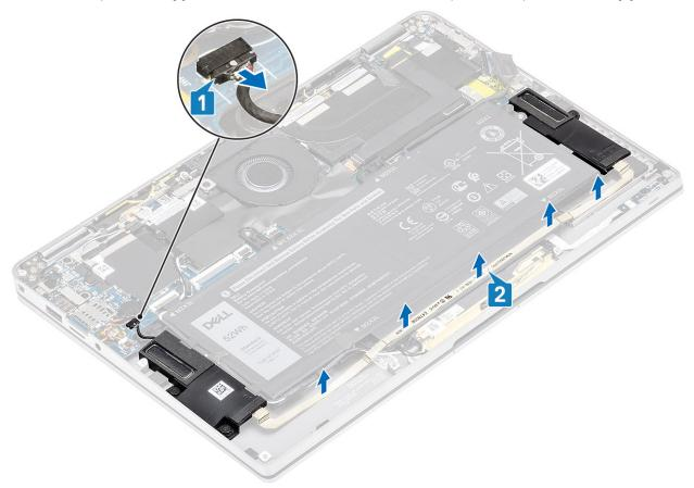
2. Remove the three (M1.6x1.4) screws [1] that secure the speakers to the system board and lift the speakers off the computer [2].
