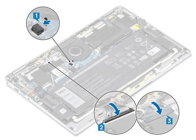
$\textbf{8.} \quad \text{Adhere the Mylar sheet on the system board.}$
