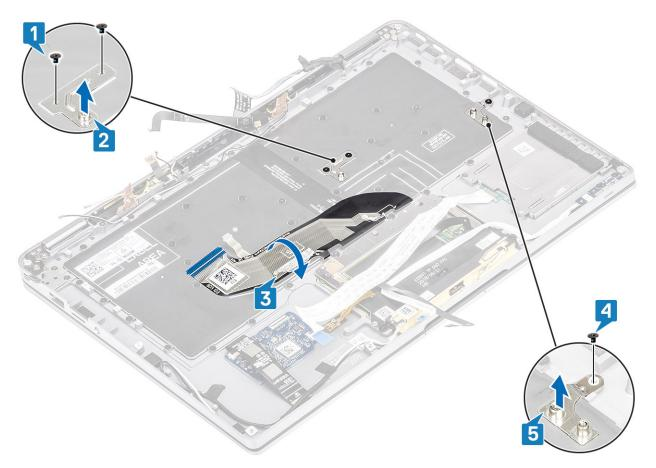
7. Remove the 40 (M1.6x1.5) screws that secure the keyboard to the palmrest assembly. Several of the screws are covered by the touchpad flexible flat cable, LED flexible flat cable (FFC), keyboard flexible printed circuit (FPC), and copper foil. Technicians must peel back these FFC/FPC/foil in order to access the keyboard screws.
