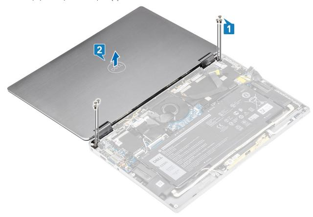
NOTE: The display assembly is a Hinge-Up Design (HUD) assembly and cannot be further disassembled once it is removed from the bottom chassis. If any components of the HUD assembly are malfunctioning and need to be replaced, replace the entire display assembly.
