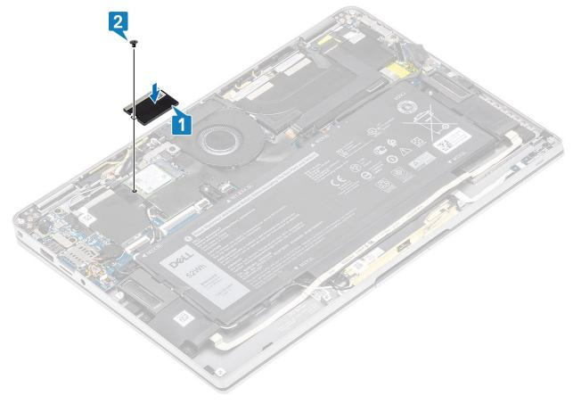
3. Affix the black tape [1] and the metal foil [2] to secure the SSD shield in place.
