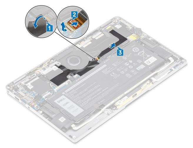
**4.** Remove the metal foil from the heatsink shield.
