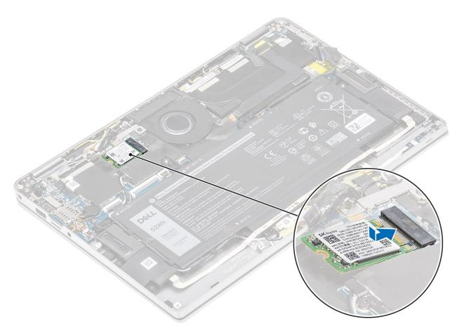
$\textbf{2.} \quad \text{Place the SSD shield on the SSD module [1] and replace the single (M2x2) screw [2] to secure it to the system board.}$
