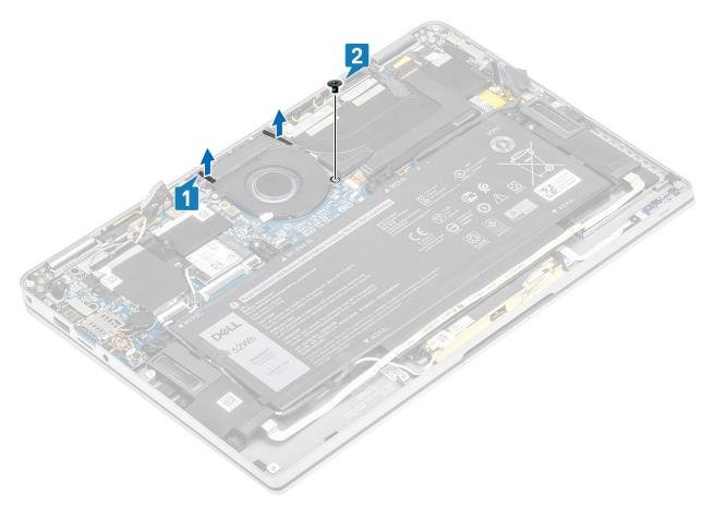
8. CAUTION: There are cushions, partially obstructing the palmrest, on the bottom side of the fan. Technicians should not lift the fan directly up, as it may damage the fan.
