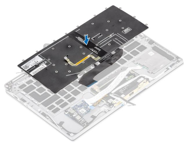
2. Replace the 40 (M1.6x1.5) screws on the keyboard to secure it to the palmrest assembly. Several of the screws are covered by the touchpad flexible flat cable, LED flexible flat cable (FFC), keyboard flexible printed circuit (FPC), and copper foil. Technicians must peel back these FFC/FPC/foil in order to access the keyboard screws.
