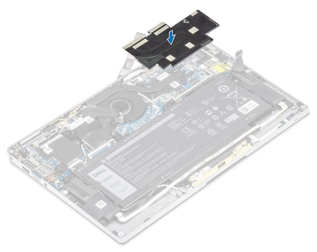
**4.** Adhere the metal foils on the heatsink shield.
