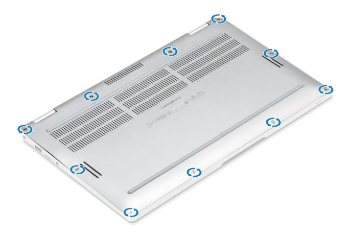
2. Pry the base cover along the edges from the top side [2] to separate the base cover from the computer [2].
