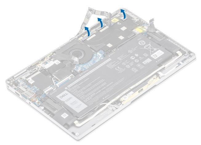
$\textbf{5.} \ \ \text{Remove the heatsink shield from the system board}.$
