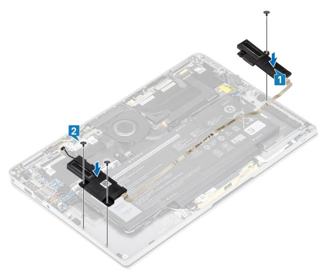
3. Connect the speaker cable [1] to the connector on the system board and adhere the speaker flex cable [2] on the battery.
