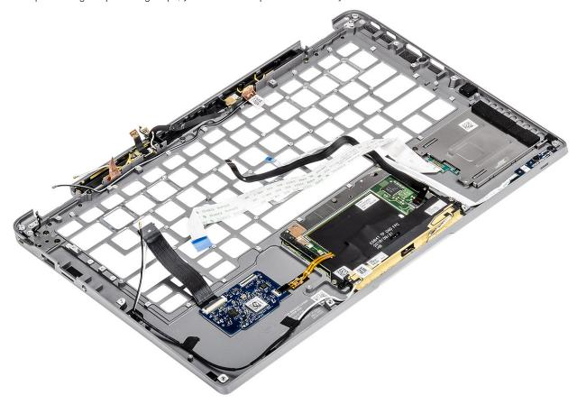
2. Transfer the post-requisite components onto the new palmrest assembly.
