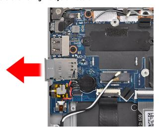
Remove the five (M2x3) screws [1] and remove the system board from the computer [2].
