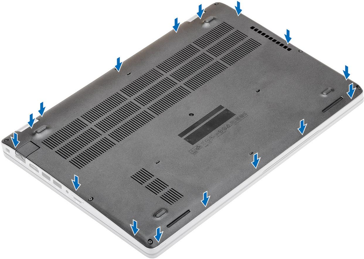
3. Tighten the eight captive screws to secure the base cover to the computer.
