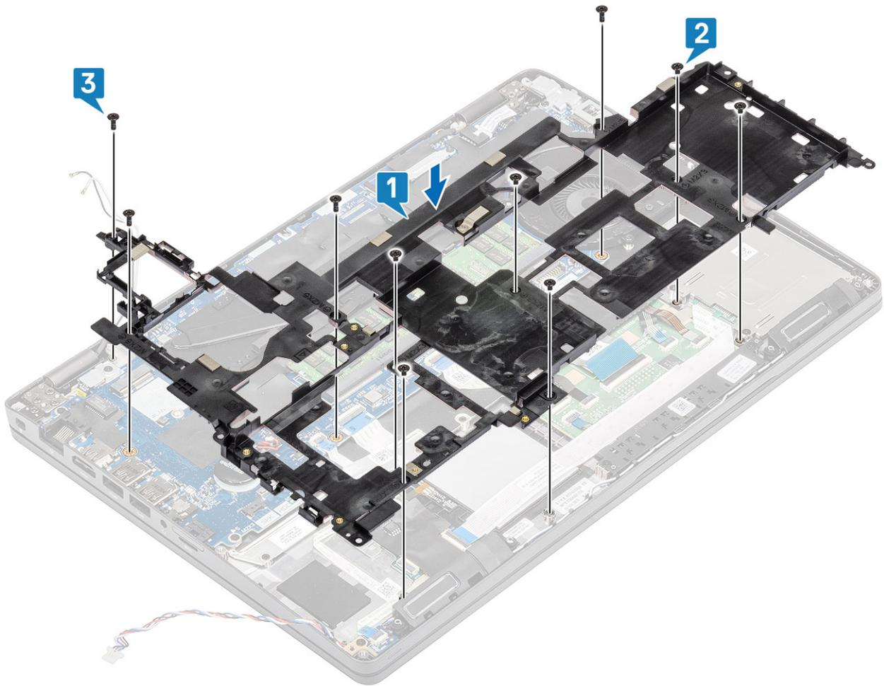
3. Re-route the wireless antennas and the speaker cable through the routing clips [1,2].
