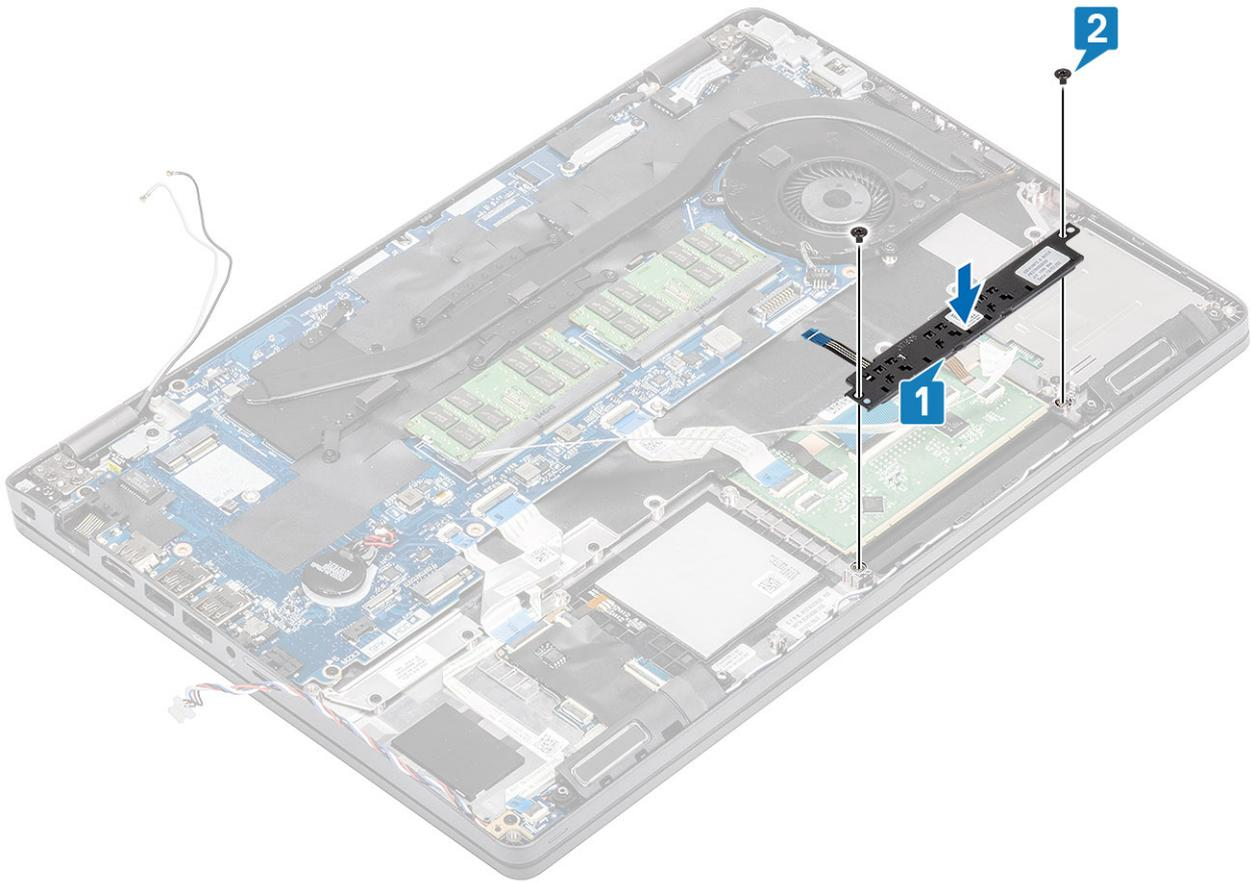
3. Re-connect the smart card reader cables and press it down to the computer chassis [1,2].
