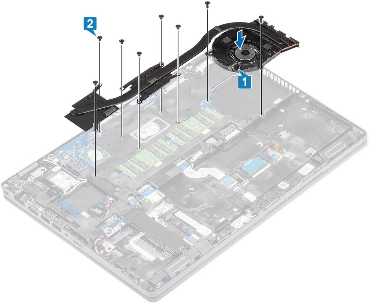
3. Re-connect the Heatsink fan cable to the connector on the system board.
