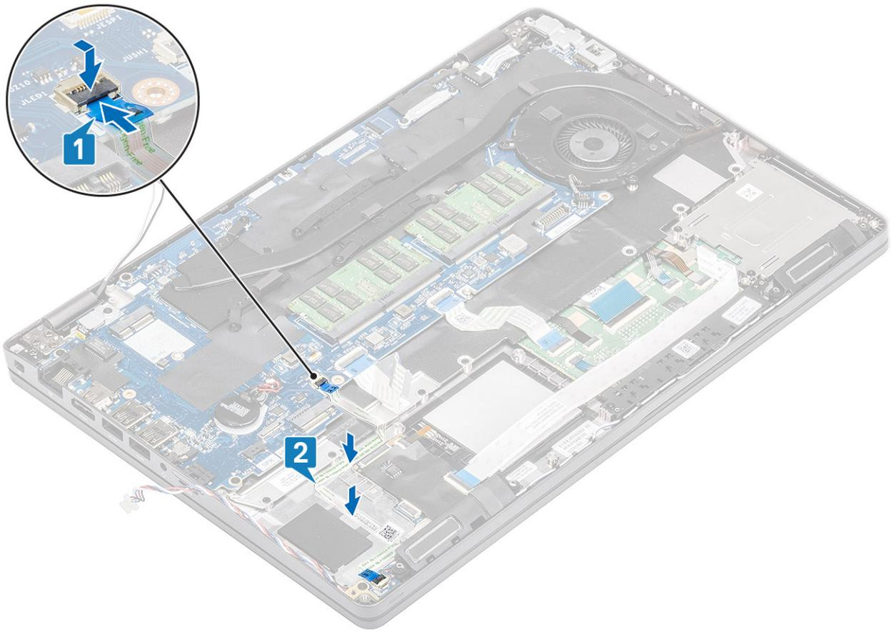
3. Gently fold the fold the USH cable as shown [1].
