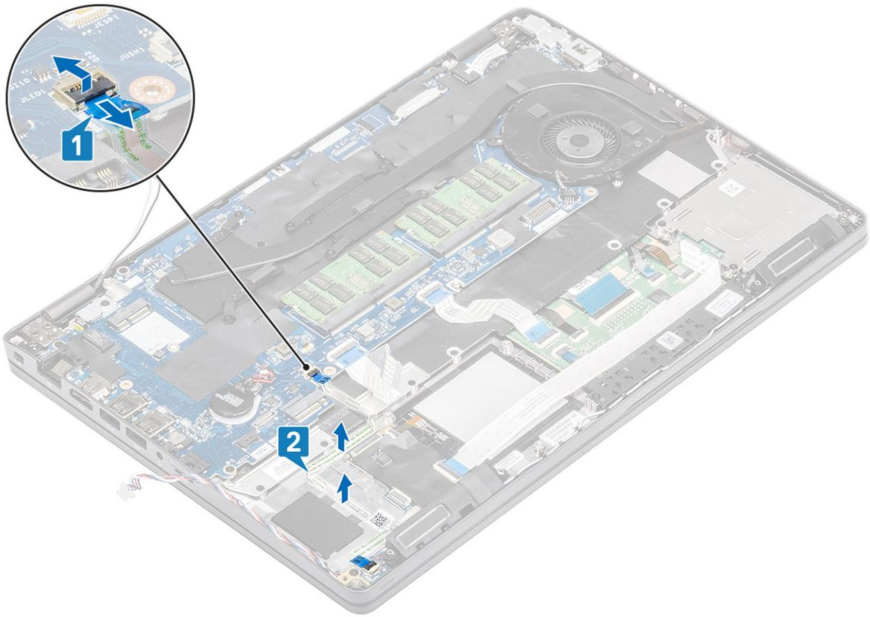
4. Remove the single (M2x2.5) screw and lift the LED board out of the computer [1,2].
