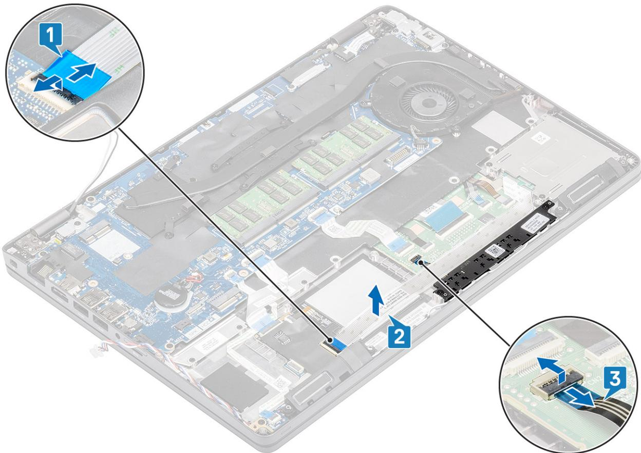
3. Remove the two (M2x3) screws and lift the touchpad away from the computer [1,2].
