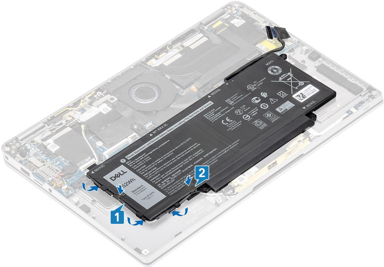
5. Connect the battery cable to the system board.
