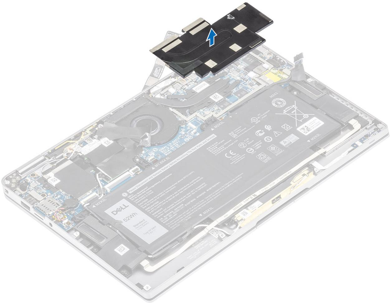
6. Remove the four (M1.6x2.5) screws [1] that secure the heatsink on the system board.
