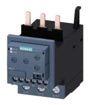
Monitoring relay, can be mounted to Contactor 3RT2, Size S2 basic, analog adjustment Apparent current monitoring 8...80 A, 50...60 Hz, 2-phase Supply 24-240 V AC/DC 1 change-over contact Monitoring for Current overshoot and undershoot Phase failure, Cable break with or without fault buffer ON delay 0-60 s Noise pulse suppression 0-30 s Switching hysteresis 6% Screw connection system
