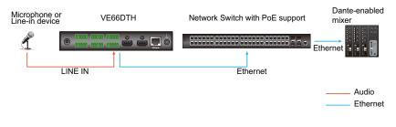
Note: The VE66DTH is used to integrate up to 6 analog LINE signals into a Dante™ networking system.
