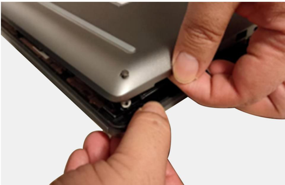
3. Lift the base cover starting from the bottom edge and remove it from the computer.
