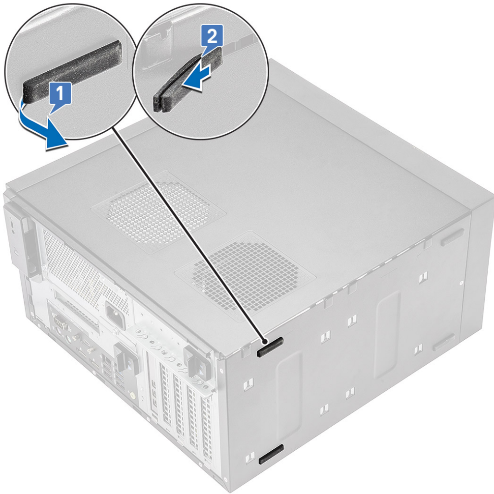
Figure 5. Rear rubber feet removal
