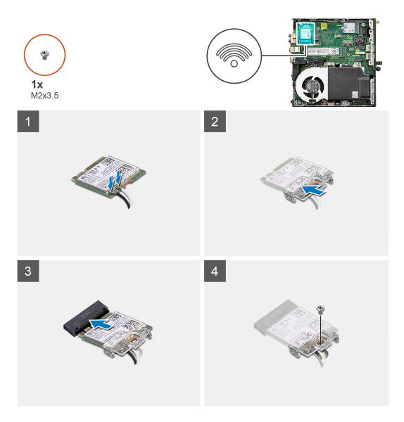
1. Connect the antenna cables to the WLAN card.
