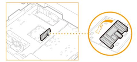
2 Lift up the lock lever (ⓐ) on the front guide, and slide it backwards or forwards to align it with the groove marked with the desired paper size.
