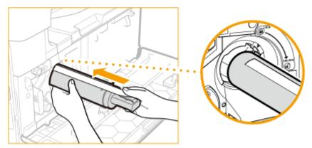
**7** Hold the toner cartridge in place with one hand, and then remove the protective seal by pulling it straight out with the other hand.
