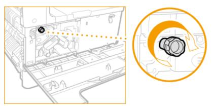
**1** Slowly turn the lock release lever to the vertical position.
