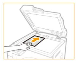
• Align the corner of the original with the top-left corner of the platen glass.
