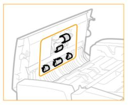
**4** Clean the inside of the inner cover of the feeder.
