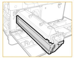
8 Wrap your hand as shown in the diagram while supporting the protective cover (1) and push the drum unit into the machine (2).
