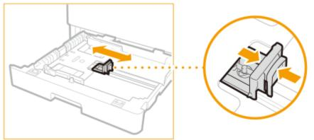
2 While squeezing the top part of the front guide, slide it to align with the size indicator for the paper to be loaded.
