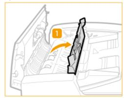
1 Open the inner cover of the feeder.
