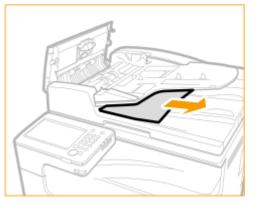
**4** Check whether an original is jammed inside the inner cover of the feeder.
