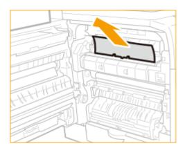
**4** Remove any jammed paper that is protruding from the upper and lower parts of the duplex unit.
