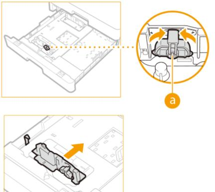
**3** Lower the lock lever to lock the front guide into place.
