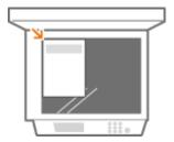
• Place the test page so that the side with the printed stripes is face down and the stripes on the page are located on the far side of the machine.
