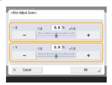
• Set the magnification of <X> for horizontal width adjustment, and the magnification of <Y> for vertical width adjustment.
