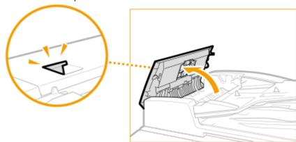
Pull the lever to open the feeder cover.
