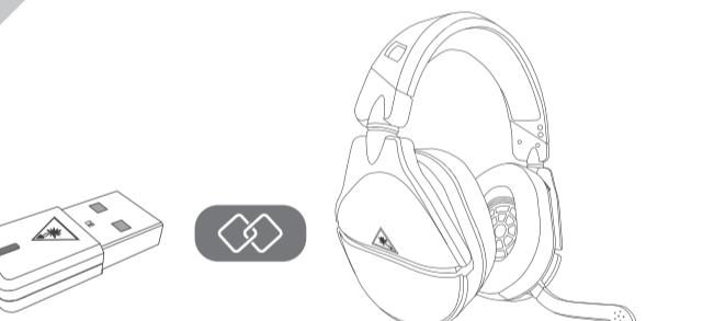
The headset and transmitter are paired out of the box, indicated by a solid LED on the transmitter. If your transmitter's LED is double-blinking, follow the steps to pair your headset and transmitter.
