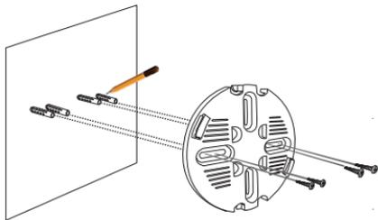
Figure 3: Attaching the Mounting Plate
