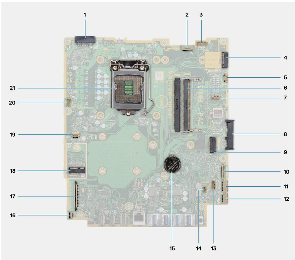
1. Power-supply unit (PSU) cable connector
