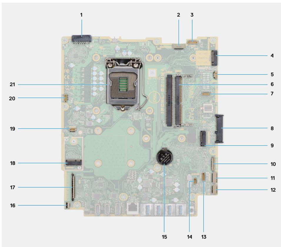
1. Power-supply unit (PSU) cable connector
