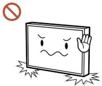
Do not stand the product as shown in the image. The panel is fragile and can get damaged.
