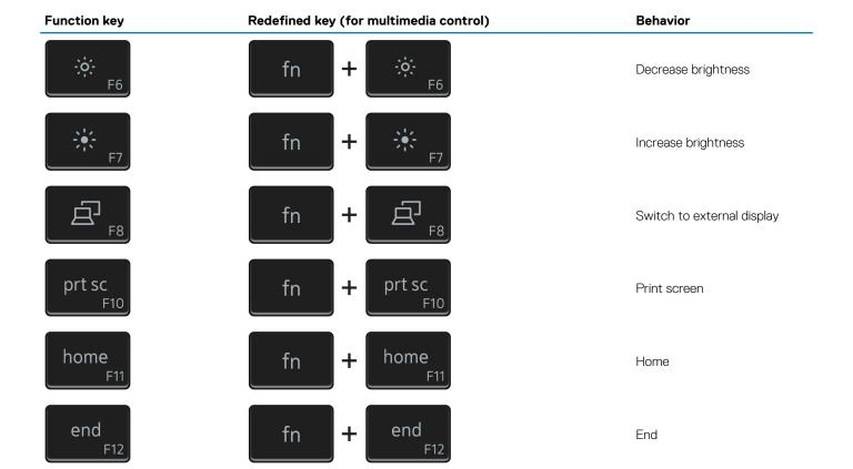
The  $\mathbf{Fn}$  key is also used with selected keys on the keyboard to invoke other secondary functions.
