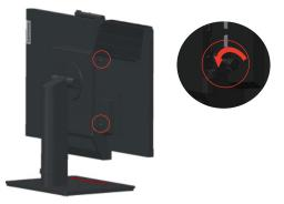
2. Push the computer from the rear as shown to disconnect it completely from the 3 in 1 cable.
