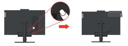
2. Pivot the rear Wi-Fi antenna downward at an angle of about 90°. Then, hold the thicker end of the rear Wi-Fi antenna and unscrew it from the computer.
