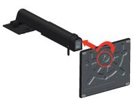
3. Insert the two metal tabs on the stand into the corresponding holes on the rear of the monitor. Then, pivot the stand downward until it clicks into position.
