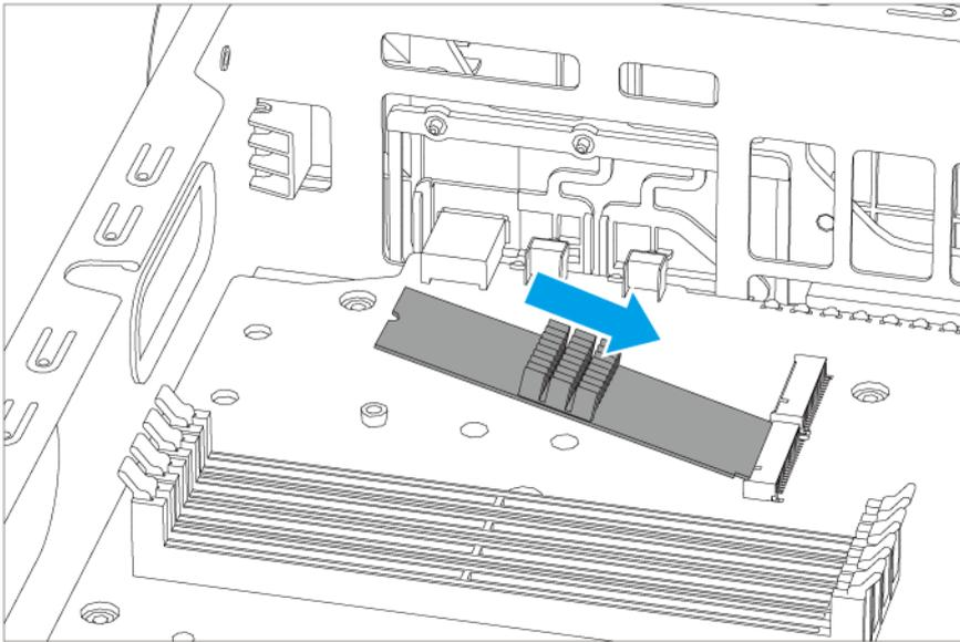
c. Insert the pushpin to secure the drive.
