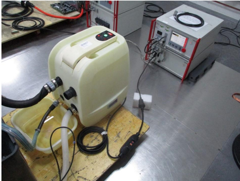
Photograph 7: Set-up for immunity of injected current
