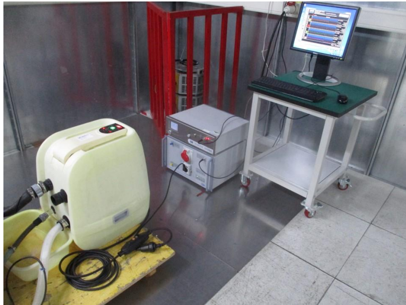
Photograph 4: Set-up for measurement of disturbance power
