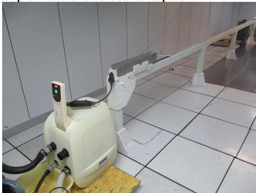
Photograph 4: Set-up for measurement of disturbance power
