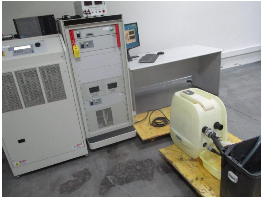
Photograph 2: Set-up for measurement of disturbance voltage
