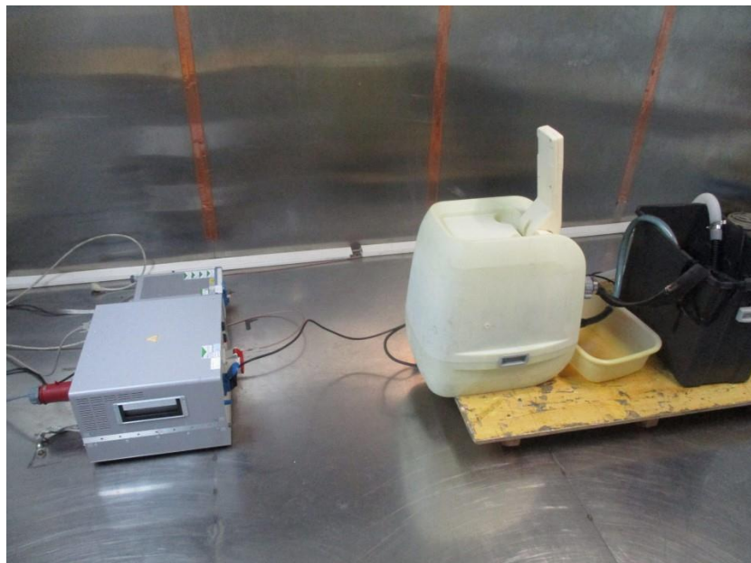
Photograph 2: Set-up for measurement of disturbance voltage
