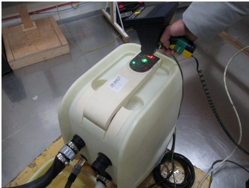
Photograph 5: Set-up for immunity of ESD
