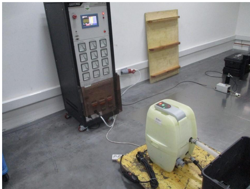
Photograph 7: Set-up for immunity test of voltage dips and short interruptions
