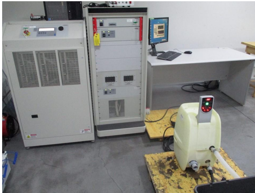
Photograph 2: Set-up for measurement of disturbance voltage on AC mains
