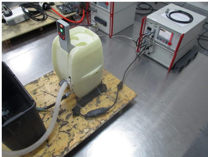
Photograph 5: Set-up for immunity test of fast transient/burst and surge
