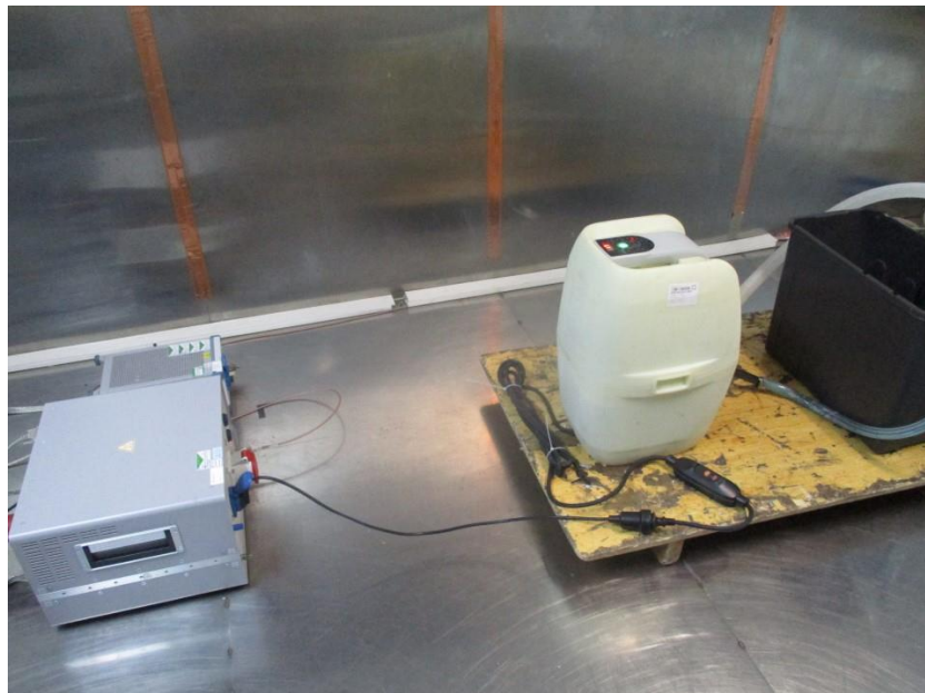
Photograph 2: Set-up for measurement of disturbance voltage on AC mains
