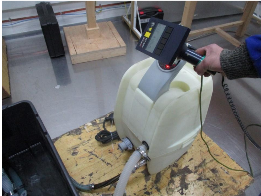
Photograph 4: Set-up for immunity test of RF electromagnetic field
