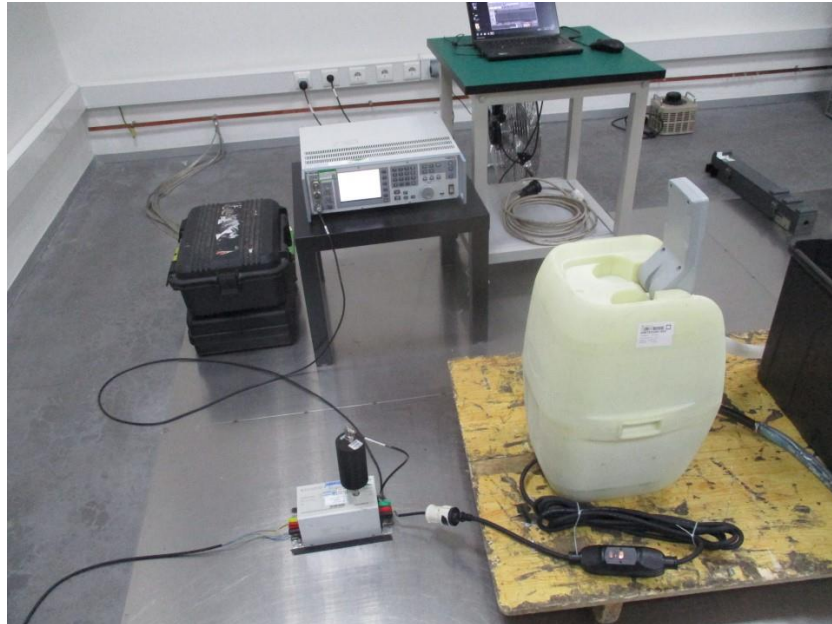
Photograph 7: Set-up for immunity test of voltage dips and short interruptions
