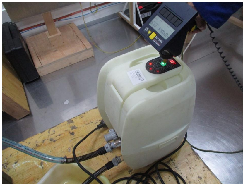
Photograph 5: Set-up for immunity of ESD
