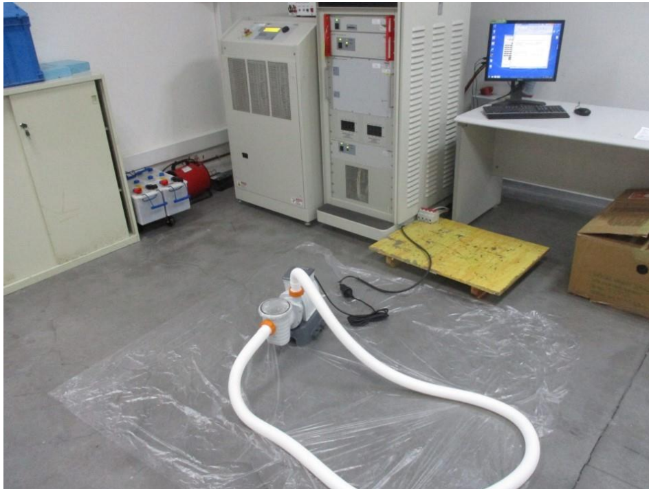
Photograph 1: Set-up for measurement of harmonics and voltage fluctuation
