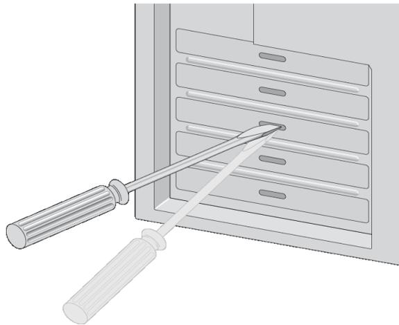
Figure 10. Removing the Faceplate From PCIe Slot
