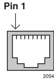
Figure 58. Pin Layout (Front View) of the Twisted Pair Port on the DNC10T Adapter
