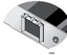
Figure 4. SFP+ Port on the DNC10SP Adapter
