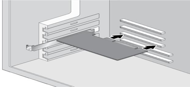
Figure 11. Inserting the Network Adapter
