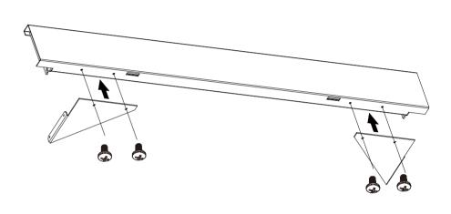
Step 2. Connect each of 6 beams to the rear door with 2 screws.
