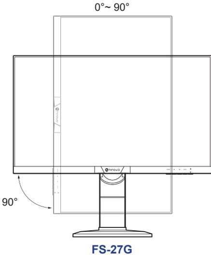
**Note:** Before making the adjustment, make sure to adjust the height to the highest position, and then tilt the screen 90°.
