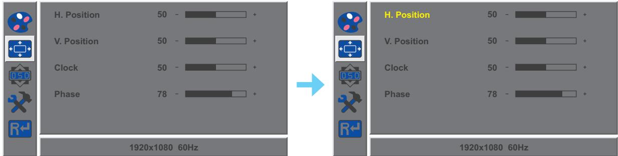
3. Press the ◀ or ▶ button to select an option and press the MENU button to enter its submenu.
