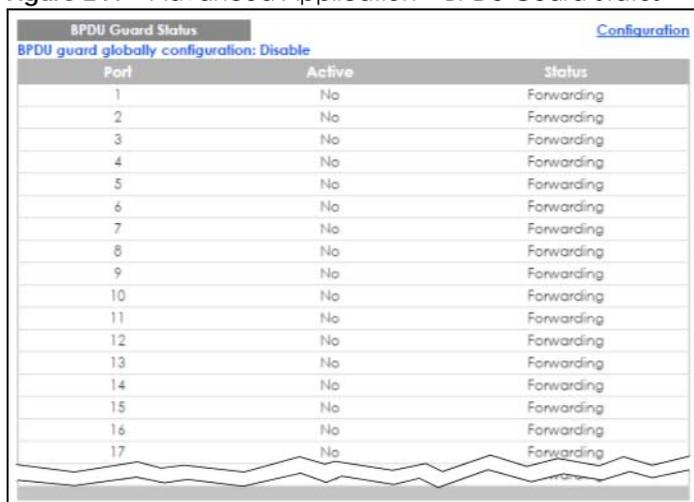
The screenshot shows the 'BPDU Guard Status' screen. At the top, there is a 'Configuration' link. Below it, the text 'BPDU guard globally configuration: Disable' is displayed. The main content is a table with three columns: 'Port', 'Active', and 'Status'. The table lists ports 1 through 17. All 'Active' values are 'No' and all 'Status' values are 'Forwarding'.
