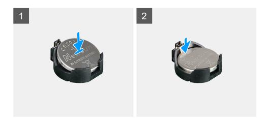
With the positive-side facing up, insert the coin-cell battery into the battery holder on the system board and gently press the battery until it snaps into place.
