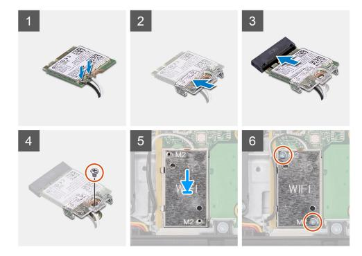
Connect the antenna cables to the wireless card.
