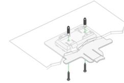
2. Hold the access point upside down with the front of the access point facing the bracket. Then, line up the guides on the bottom of the access point with the bracket.
