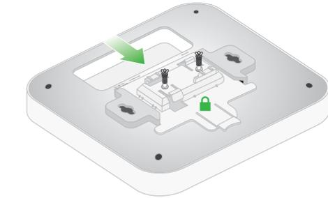
**Note:** To unlock the access point, push the locking tab toward the ceiling and slide the access point out of the bracket.
