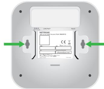
1. Mark the wall where you want to insert the provided anchors and screws, which must be 3.875 in. (98.5 mm) apart, and insert the anchors and screws.
