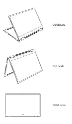
**NOTE:** Rotating the screen to Stand, Tent and Tablet mode will disable the keyboard and touchpad.
