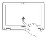
Slide your fingertip upward from the bottom edge of the screen to toggle on and off the auto-hide shelf
