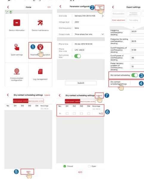
Figure B-1 Setting dry contact scheduling parameters
