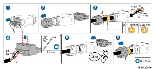
Figure 5-7 Four-core cable (L1, L2, L3, and PE)
