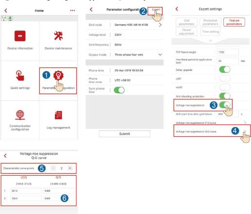
Figure D-1 Setting voltage rise suppression Q-U curveparameters
