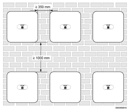
Figure 4-5 Stacked installation (not recommended)
