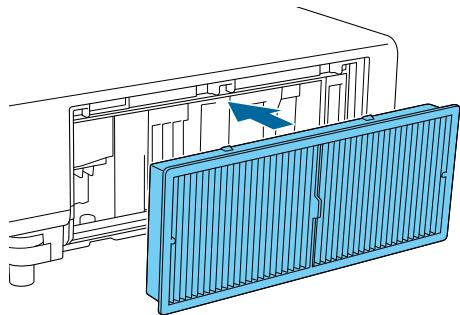
**6** Close the air filter cover and tighten the fixing screws.
