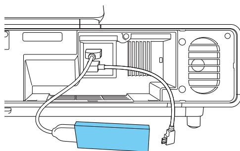
6 Connect the USB power cable to the USB port (type B) on the streaming media player.
