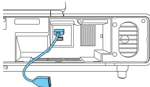
4 Connect the USB power cable supplied to the DC Out (2.0A) power supply port.
