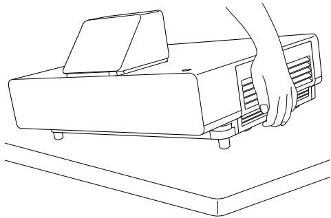
**3** Loosen the fixing screws and open the air filter cover.
