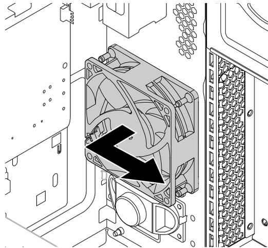
*Figure 122. Removing the front fan*
