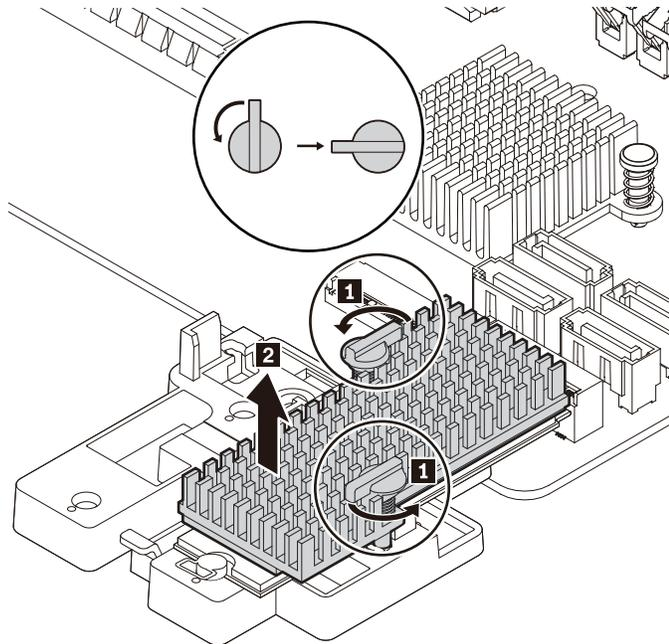
Figure 35. Removing the heat sink from the plastic holder
