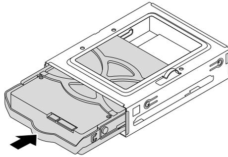
Figure 99. Installing the storage drive
