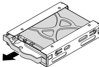
Figure 110. Removing the 2.5-inch storage drive
