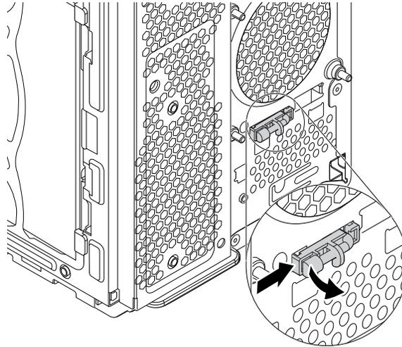
Figure 127. Removing the thermal sensor
