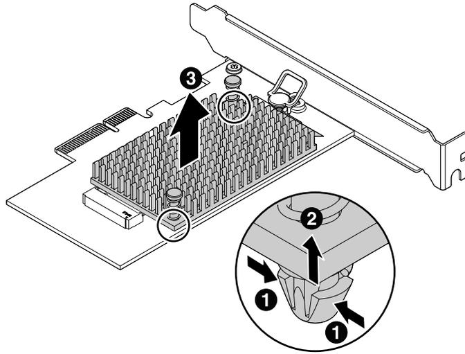
Figure 42. Removing the heat sink from the M.2 solid-state drive adapter
