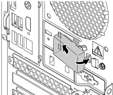
Figure 149. Installing the shield
