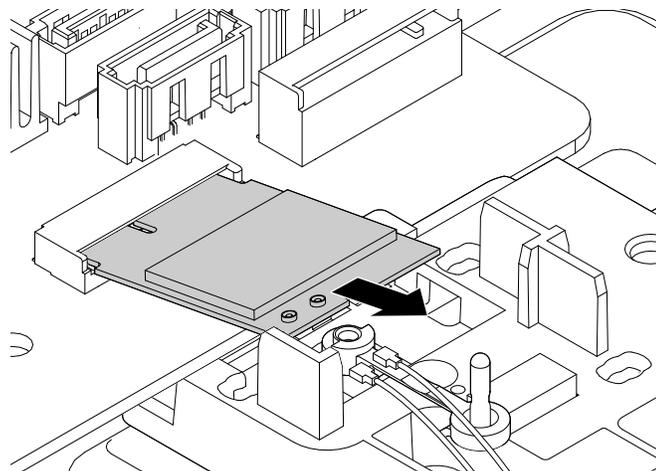
*Figure 133. Pulling the Wi-Fi card module out of the Wi-Fi card slot*
