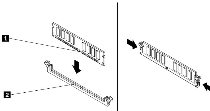
Figure 50. Installing a memory module
