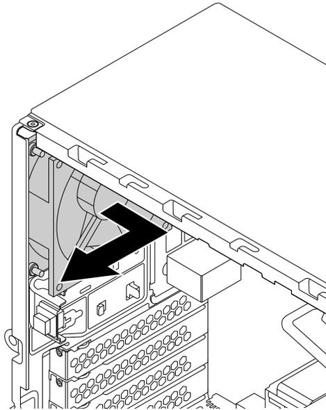
Figure 124. Removing the rear fan
