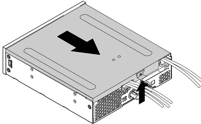
Figure 168. Removing the flex module cover
