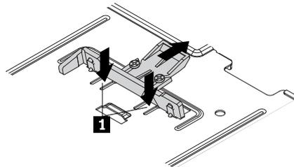
Figure 160. Removing the plastic clip with the two screws
