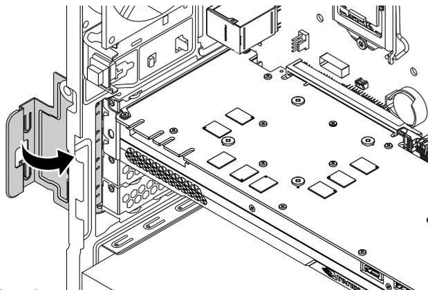
Figure 34. Rotating the PCIe card retainer
