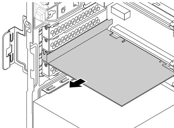
Figure 25. Removing a PCIe card
