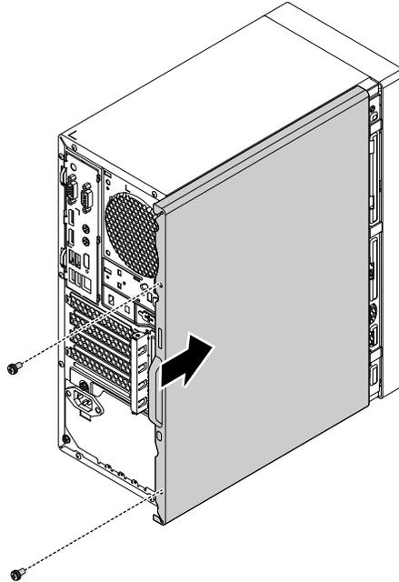
*Figure 178. Reinstalling the computer cover*
