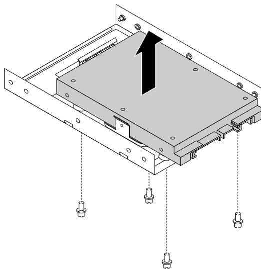
Figure 77. Removing the 2.5-inch storage drive from the storage-drive converter
