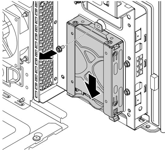
Figure 109. Removing the type-2 storage-drive cage
