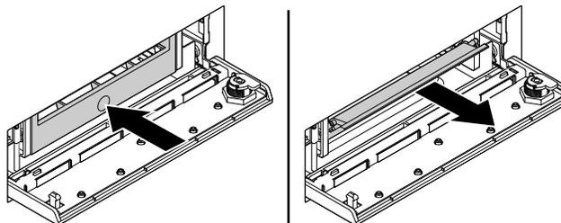
Figure 56. Removing the bracket from the front-access storage enclosure
