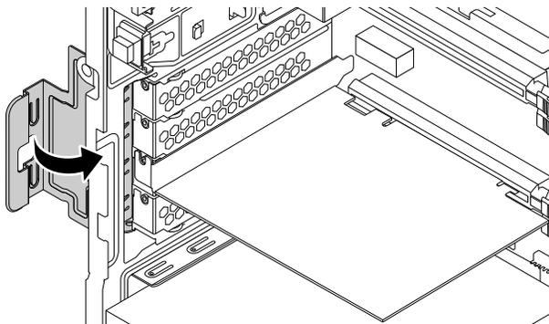
Figure 27. Rotating the PCIe card retainer
