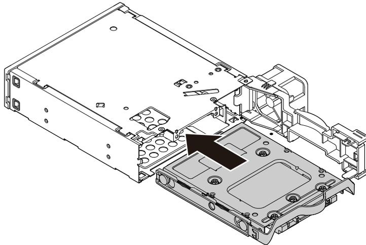
Figure 80. Installing the storage converter with the bracket into the enclosure
