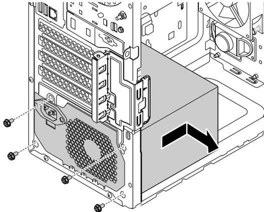
Figure 86. Removing the power supply assembly
