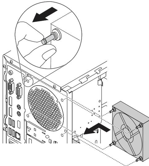
Figure 125. Installing the rear fan
