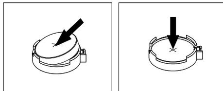
Figure 83. Installing the coin-cell battery
