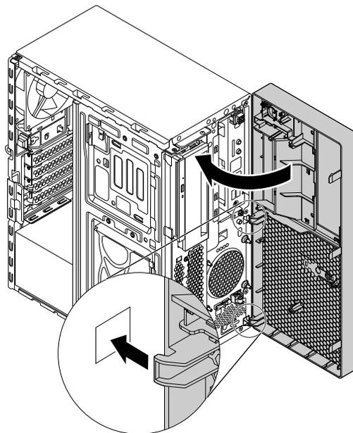
Figure 177. Reinstalling the front bezel
