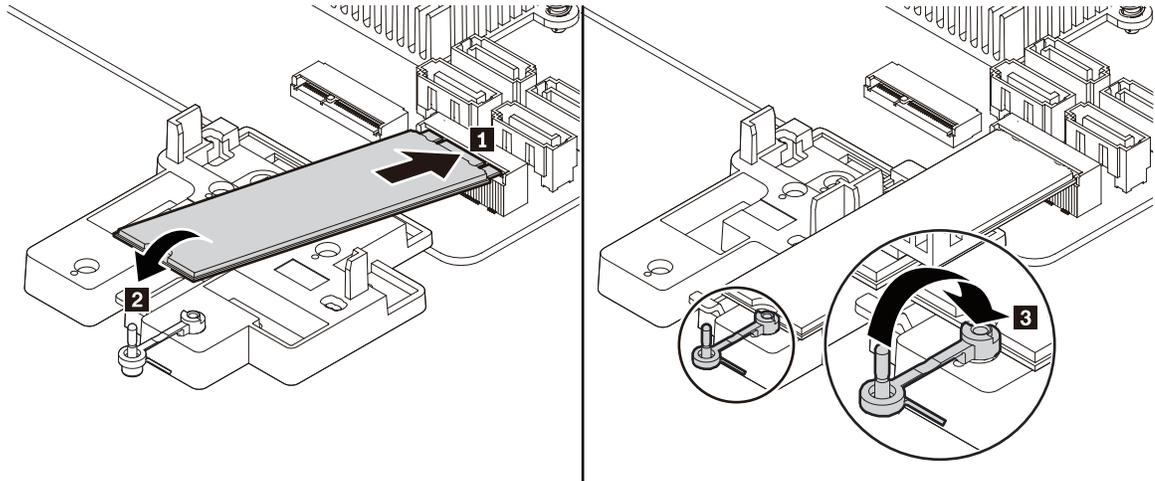
Figure 39. Installing the M.2 solid-state drive
