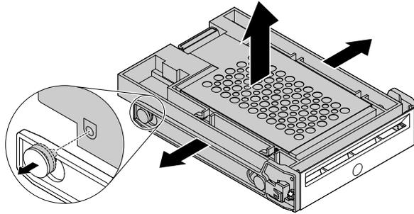
Figure 62. Removing the 2.5-inch storage drive from the bracket
