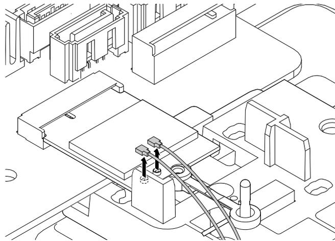
*Figure 132. Disconnecting the front and rear Wi-Fi antenna cables from the Wi-Fi card module*
