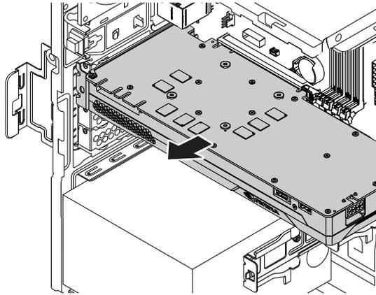
Figure 30. Removing a full-length PCIe card
