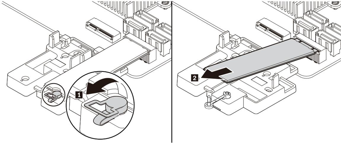
Figure 36. Opening the retention latch and removing the M.2 solid-state drive
