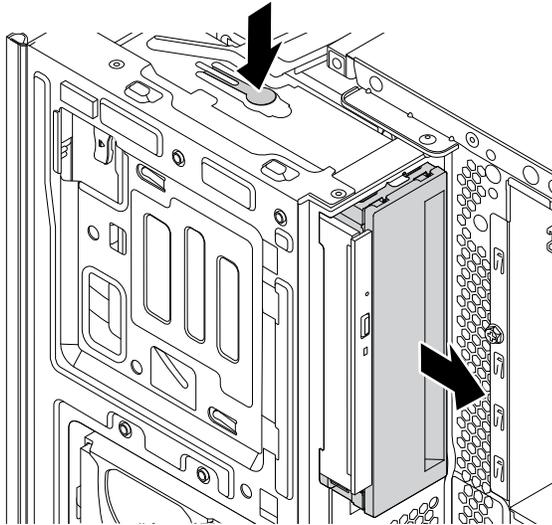
*Figure 51. Removing the flex storage enclosure*
