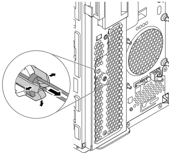
*Figure 116. Removing the ThinkStation LED*
