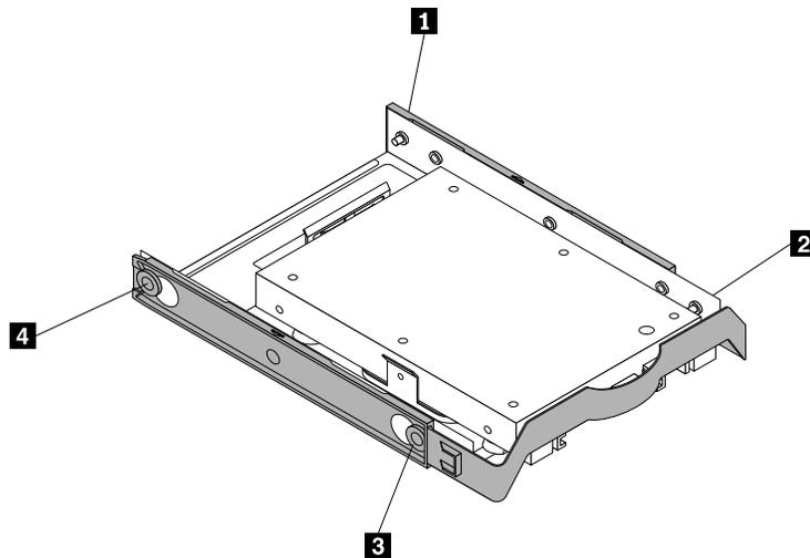
Figure 79. Installing the storage converter together with the solid-state drive into the storage drive bracket
