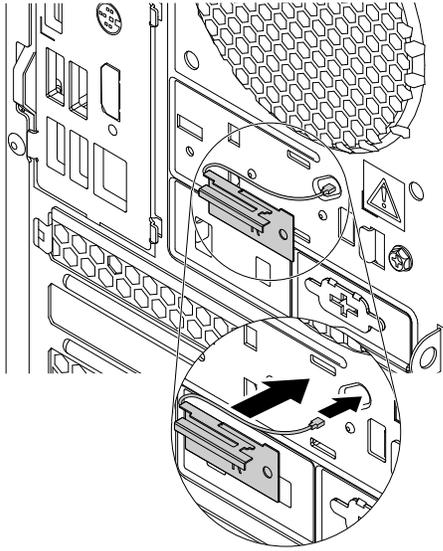
Figure 148. Installing the rear Wi-Fi antenna
