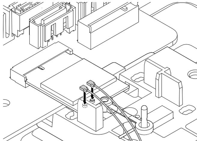
Figure 137. Connecting the front and rear Wi-Fi antenna cables to the Wi-Fi card module
