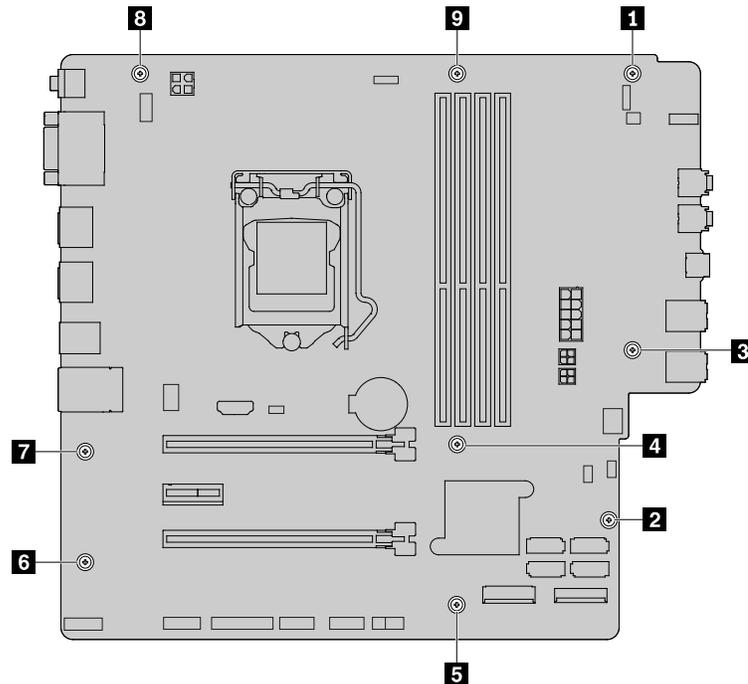
Figure 155. Installing the nine screws to secure the system board
