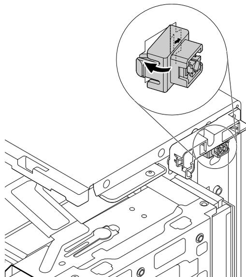
Figure 115. Installing the power button
