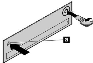
Figure 55. Opening the front-access storage enclosure cover
