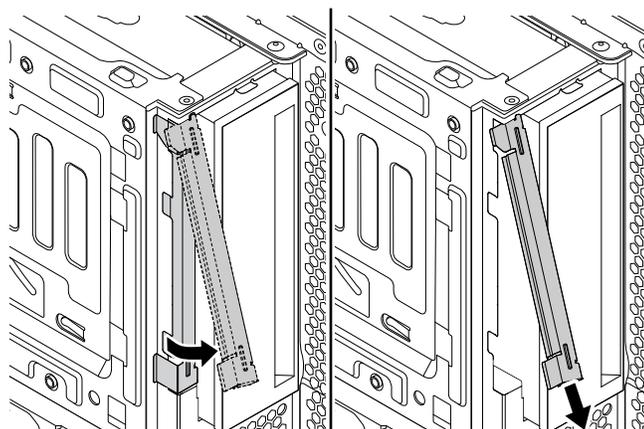
Figure 20. Removing the metal shield
