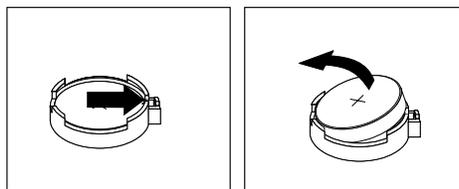
Figure 82. Removing the coin-cell battery
