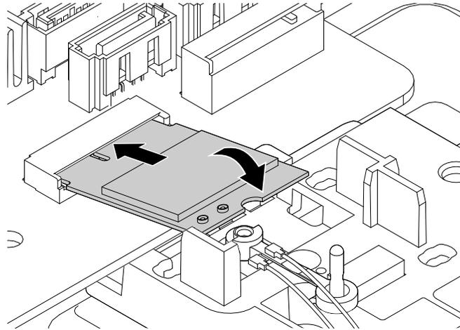
Figure 136. Installing the Wi-Fi card module
