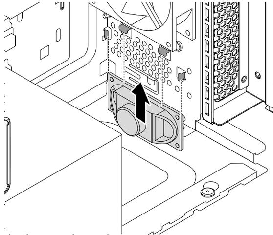
Figure 130. Installing the internal speaker
