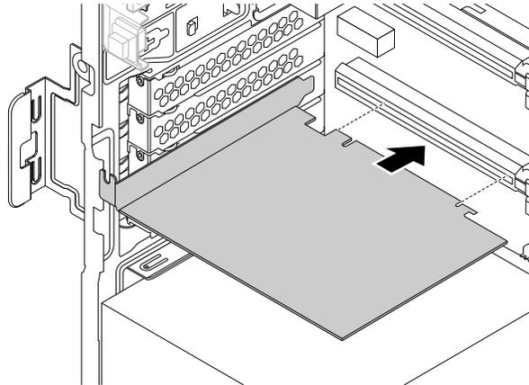
Figure 26. Installing a new PCIe card
