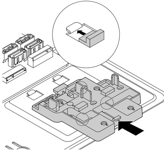
Figure 134. Installing the plastic holder
