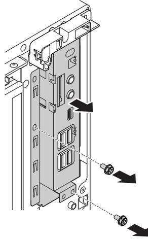
*Figure 118. Removing the front audio and USB assembly*
