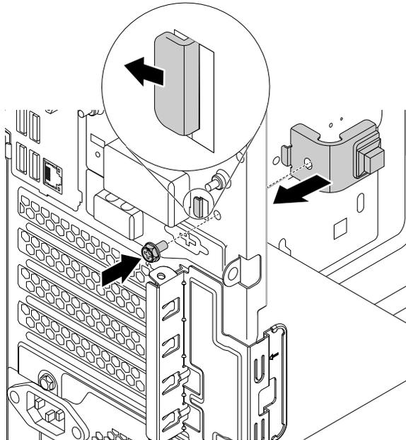
*Figure 85. Installing the cover presence switch*
