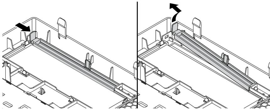
Figure 19. Removing the plastic shield
