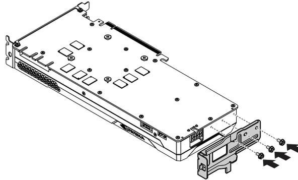
Figure 32. Installing a full-length PCIe card bracket
