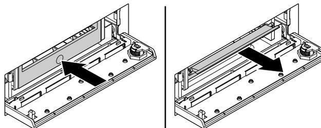
Figure 61. Removing the bracket from the front-access storage enclosure
