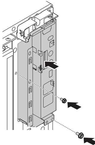
Figure 121. Installing the front audio and USB assembly
