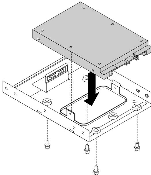
*Figure 93. Installing the new 2.5-inch storage drive into the storage-drive converter*
