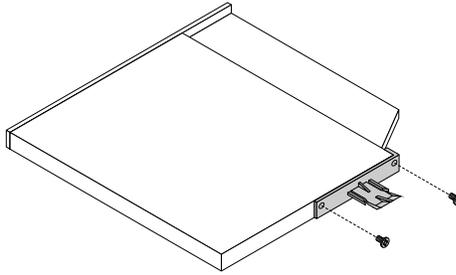
Figure 161. Installing the plastic clip to the slim optical drive
