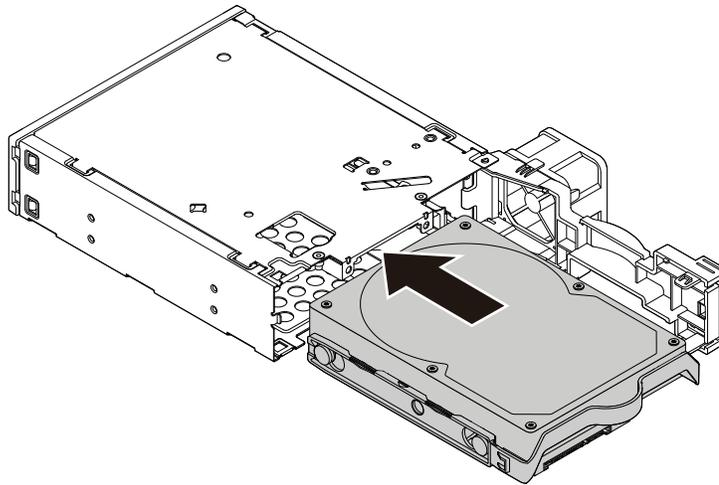
Figure 72. Installing the 3.5-inch storage drive into the enclosure
