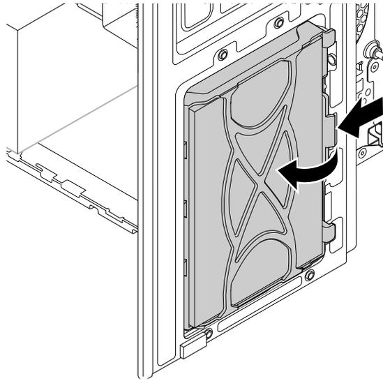
Figure 87. Removing the storage drive
