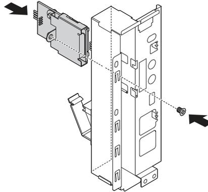
Figure 120. Installing the card reader
