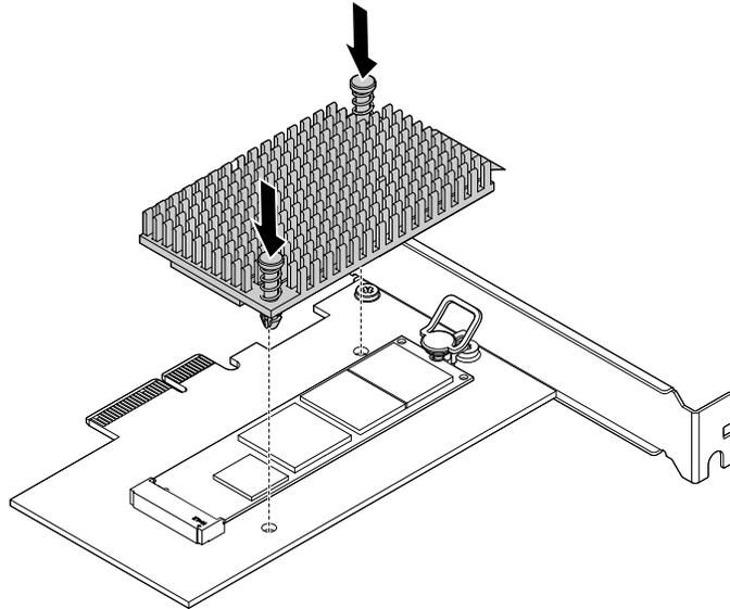
Figure 46. Installing the heat sink
