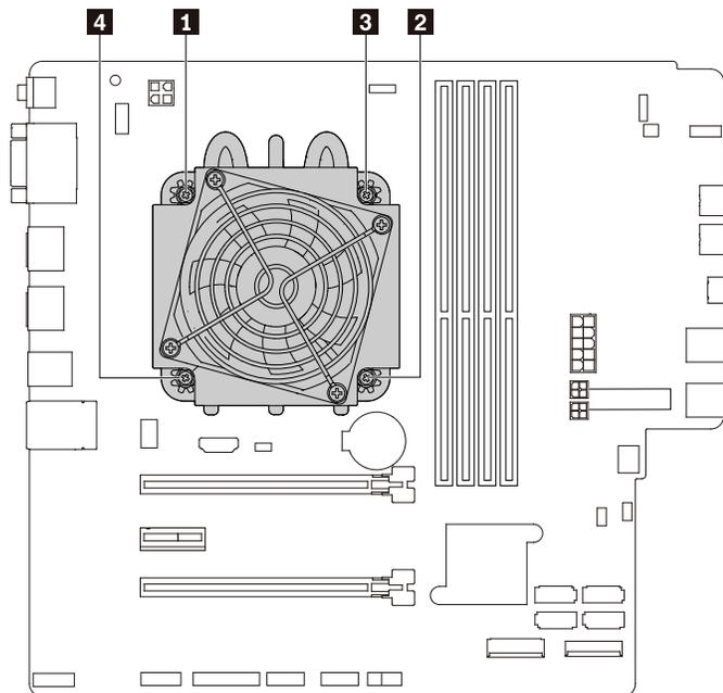
Figure 126. Removing the heat-sink-and-fan assembly
