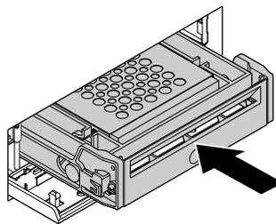
Figure 68. Installing the plastic bracket with the 2.5-inch storage drive into the front-access storage enclosure
