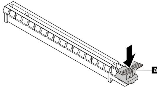
Figure 23. Disengaging the card retaining latch
