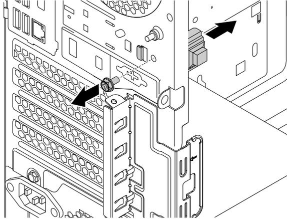
*Figure 84. Removing the cover presence switch*
