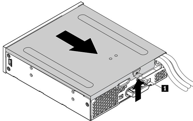
Figure 164. Removing the flex module cover
