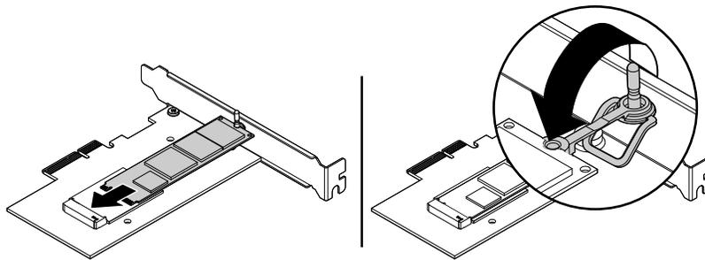
*Figure 45. Installing the M.2 solid-state drive*
