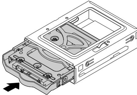
Figure 107. Installing the 2.5-inch storage drive into the type-1 storage-drive cage
