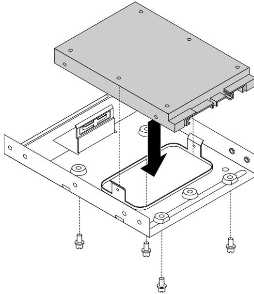
Figure 105. Installing the 2.5-inch storage drive into the storage-drive converter
