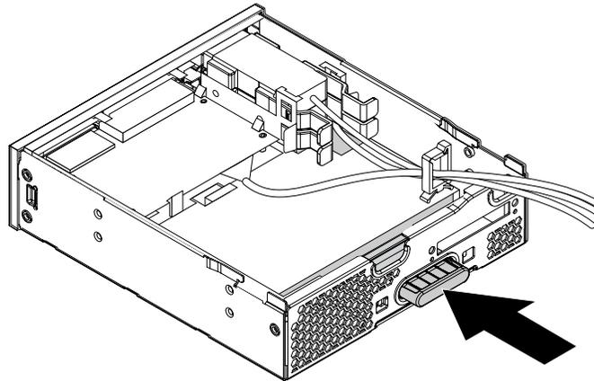
Figure 158. Removing the slim optical drive from the flex module
