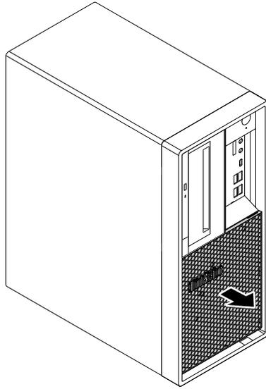
*Figure 13. Removing the dust shield*
