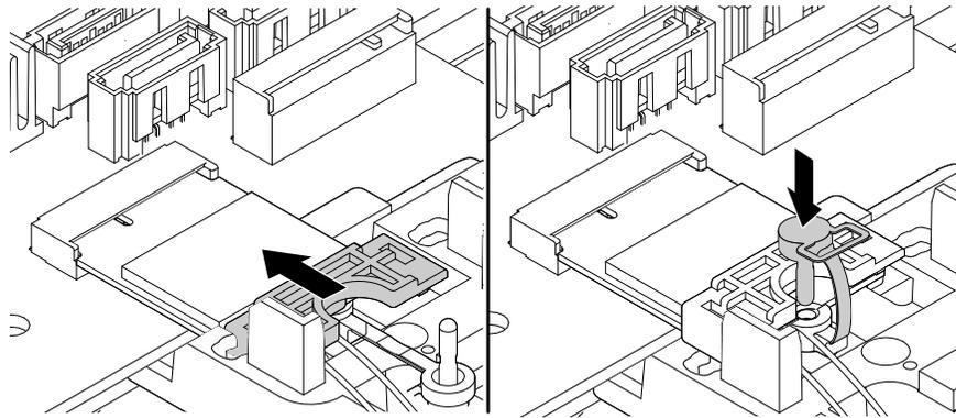
*Figure 143. Reinstalling the shield and insert the plug of the retention latch into the hole to secure the Wi-Fi card module*
