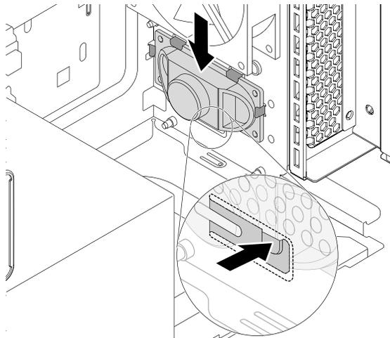
*Figure 129. Removing the internal speaker*
