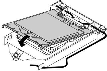
Figure 156. Installing the microprocessor socket cover
