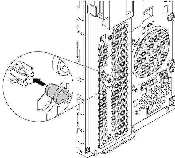
Figure 117. Installing the ThinkStation LED
