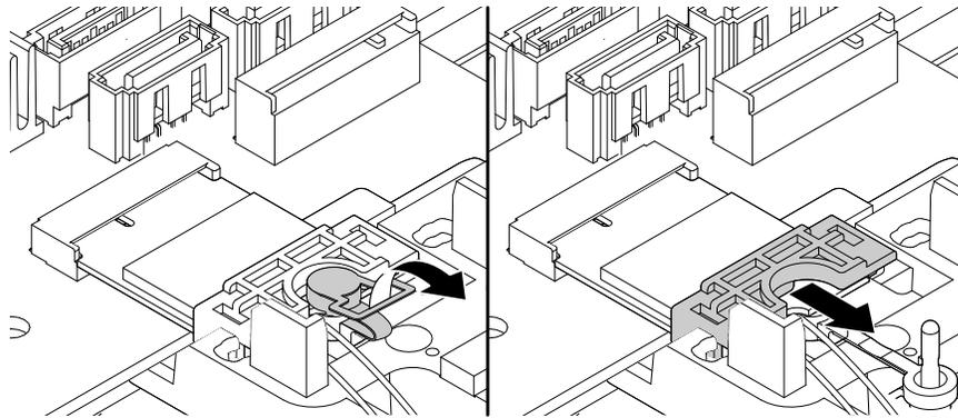
Figure 139. Pulling handle of the retention latch outward and removing the shield
