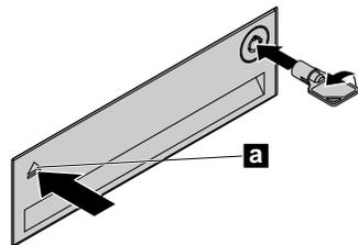
Figure 60. Opening the front-access storage enclosure cover
