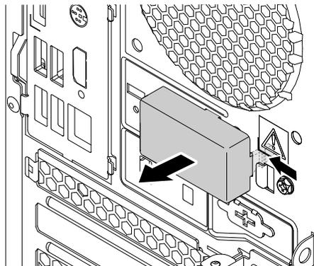
*Figure 145. Removing the shield*
