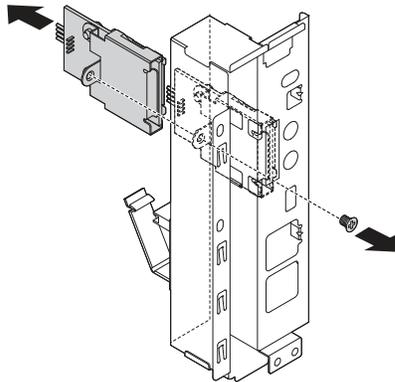
*Figure 119. Removing the card reader*
