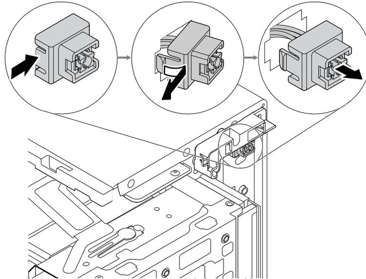
Figure 114. Removing the power button
