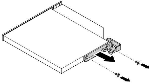
Figure 18. Removing the bracket
