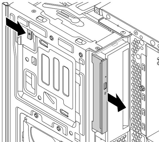
Figure 17. Removing the slim optical drive
