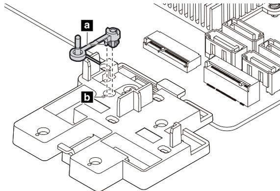
Figure 135. Installing the retention latch
