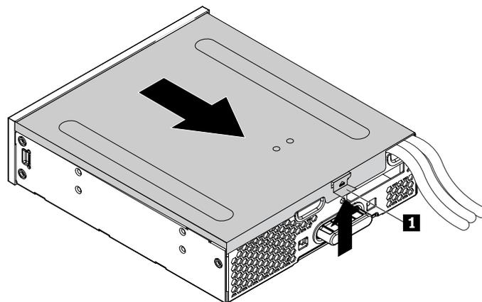
Figure 157. Removing the flex module cover
