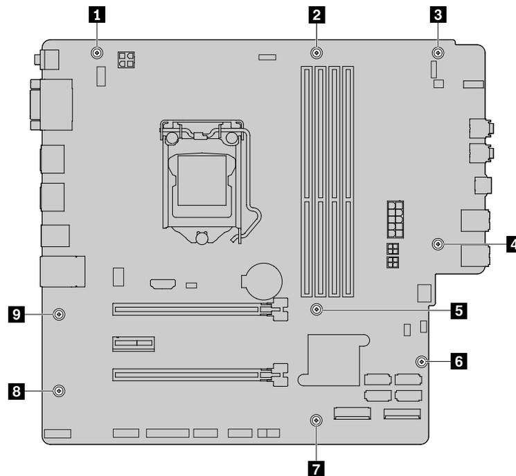
Figure 154. Removing the nine screws that secure the system board
