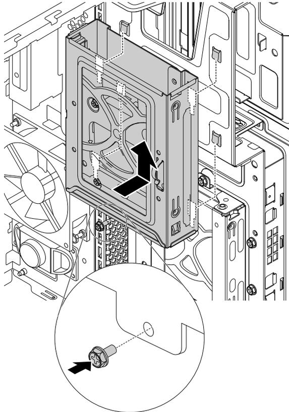
Figure 108. Installing the type-1 storage-drive cage
