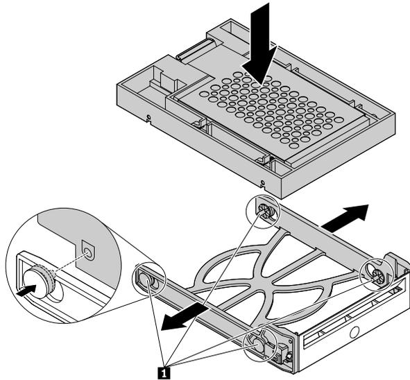
Figure 67. Installing the converter with the 2.5-inch storage drive into the plastic bracket
