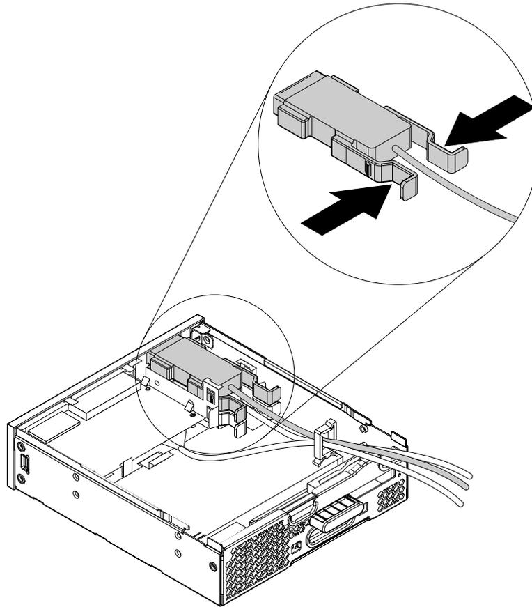
Figure 165. Removing the eSATA connector or IEEE 1394 connector from the flex module
