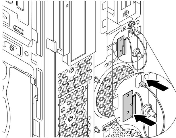
*Figure 142. Installing the front Wi-Fi antenna*
