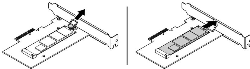
Figure 43. Removing the M.2 solid-state drive
