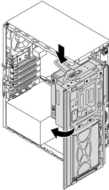
Figure 176. Pivoting the drive bay assembly downward
