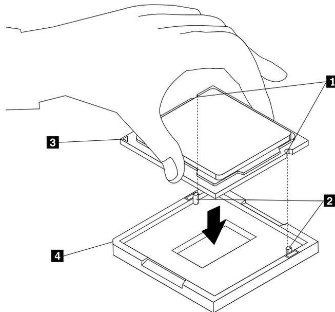
Figure 153. Installing the microprocessor
