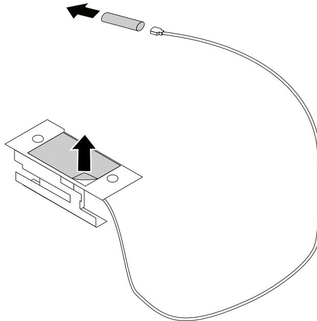
Figure 141. Peeling off the paper that protects the sticker and removing the plastic cover
