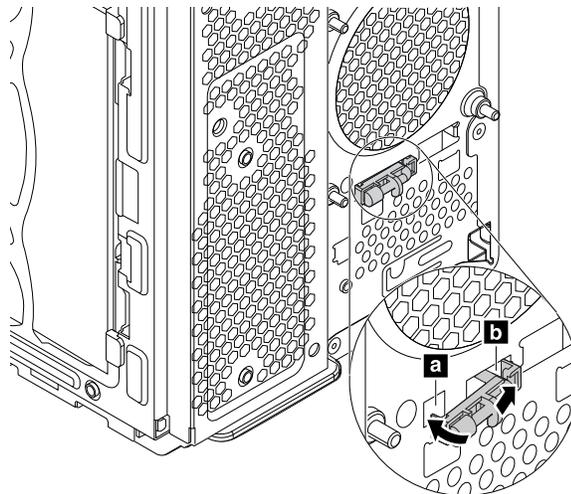
Figure 128. Installing the thermal sensor
