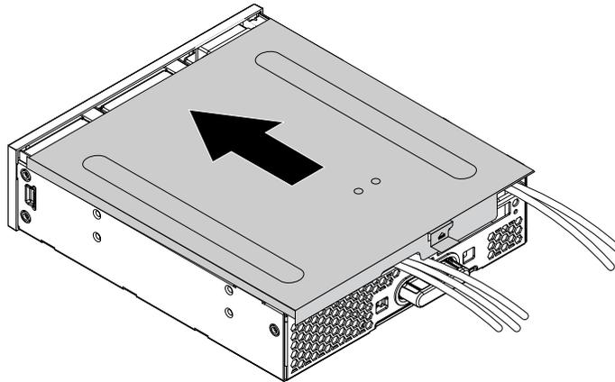
Figure 175. Reinstalling the flex module cover
