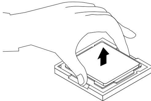
Figure 152. Removing the microprocessor
