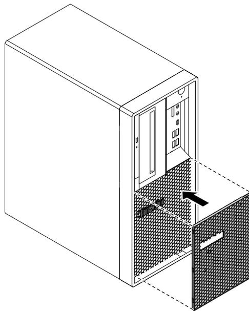
*Figure 179. Reinstalling the dust shield*
