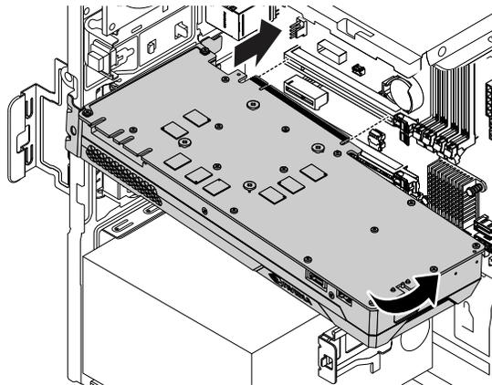
Figure 33. Installing a new full-length PCIe card
