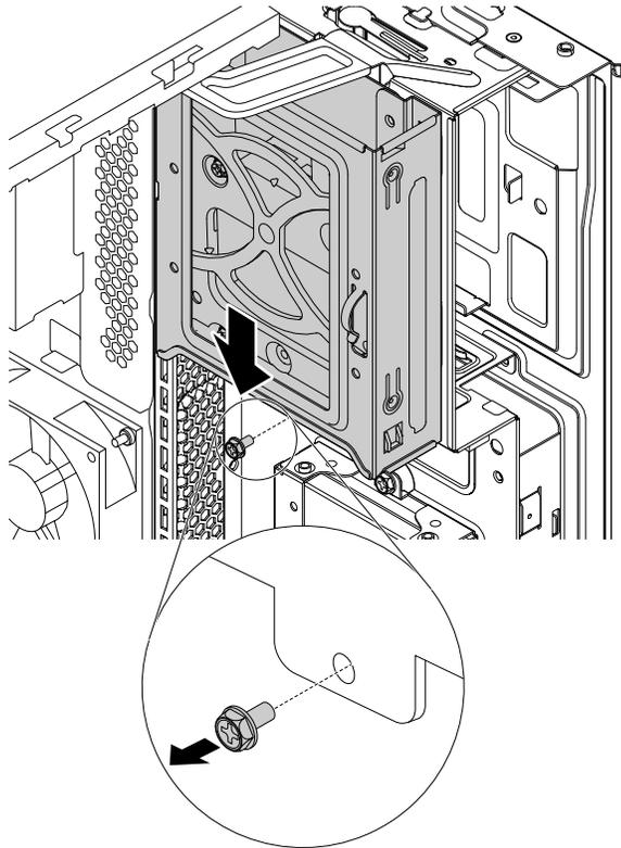
Figure 101. Removing the type-1 storage-drive cage
