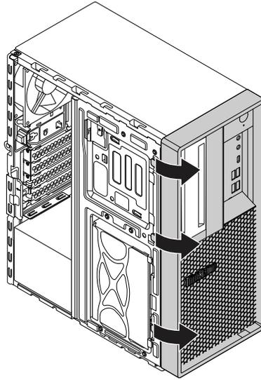
*Figure 15. Removing the front bezel*
