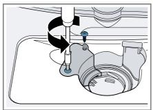
6. Pull up and remove the pump cover.
