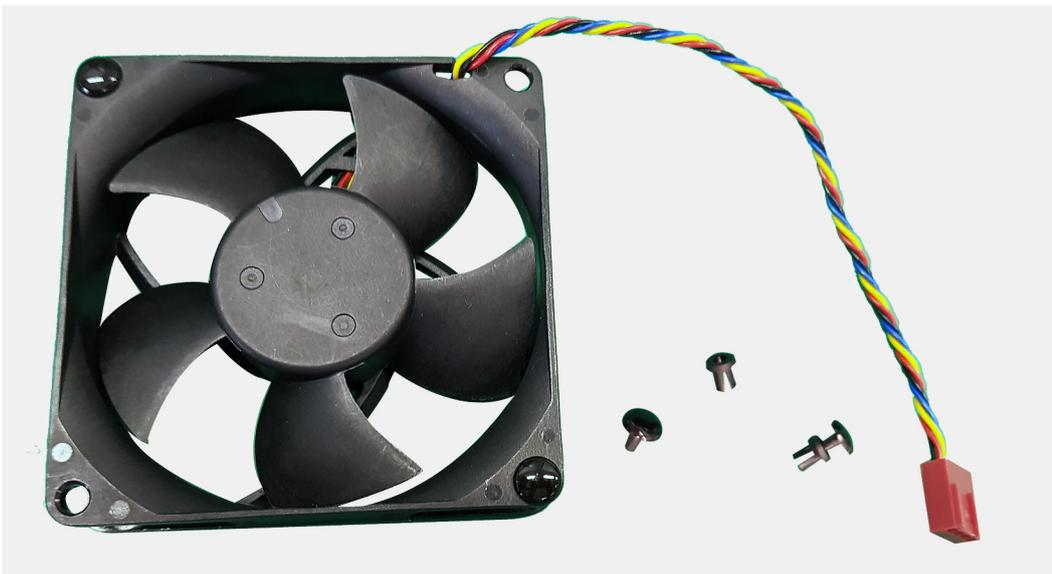
2. Route the rubber grommets through the slots on fan and pull the rubber grommets until the fan snaps into position.
