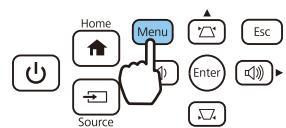
2 Use the up and down buttons to select **Quick Corner**, and then press the [Enter] button. Press the [Enter] button again if necessary.
