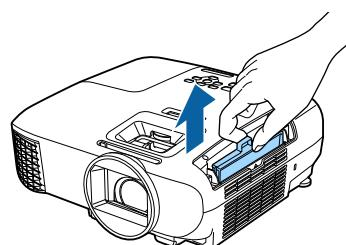
4 Hold the air filter with the surface facing down and tap it 4 or 5 times to remove the dust.
