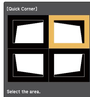
To reset the Quick Corner corrections, hold down the [Esc] button for about two seconds while the area selection screen is displayed, and then select **Yes**.
