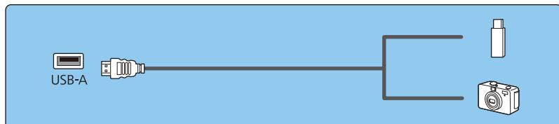
When the USB device is connected, you can project image files on the USB flash drive or digital camera as a slideshow.
