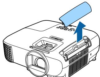
**3** Remove the air filter. Grip the air filter cover tab and pull it straight up.
