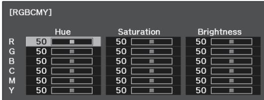
3 Use the up and down buttons to select **Hue, Saturation, or Brightness**.
