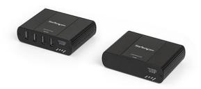
The USB2002EXT2 2-Port USB Extender lets you extend USB 2.0 devices over Cat 5 or better Ethernet cable at distances of up to 330ft (100m). A local transmitter power adapter provides up to 500 mA of power per port with no power adapter required at the remote end, letting you access and power almost any USB 2.0 device in locations where a power outlet may be unavailable.
