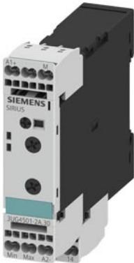
Analog monitoring relay Fill level monitoring Resistance monitoring from 2 to 200 kohm Overshoot and undershoot Supply voltage 24 V AC/DC 50 to 60 Hz DC and AC without galvanic isolation to measuring circuit 2-step or 1-step control Tripping delay 0.5 to 10 s 1 change-over contact spring-type connection system
