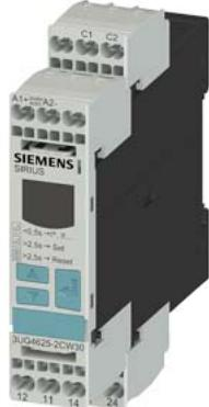
Digital monitoring relay for residual current monitoring (with current transformer 3UL23) Setting range 0.03...40 A separate for warning threshold and switch-off value supply voltage 24 ... 240 V AC/DC, 50 .. 60Hz ON delay and tripping delay 0.1 to 20 s Shutdown hysteresis up to 50% Warning hysteresis 5% fixed Width 22.5 mm, 2 change-over contacts with or without fault buffer spring-type connection system
