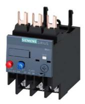
Overload relay 2.8...4.0 A Thermal For motor protection Size S0, Class 10 Contactor mounting Main circuit: Ring cable lug Auxiliary circuit: ring cable lug Manual-Automatic-Reset
