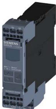
Digital monitoring relay Current monitoring, 22.5 mm for IO-Link 0.05...10.0 A AC/DC Overcurrent and undercurrent Transformer scaling factor Hysteresis 0.01 to 5.0 A ON-delay time Tripping delay time 1 change-over contact, spring-type connection system
