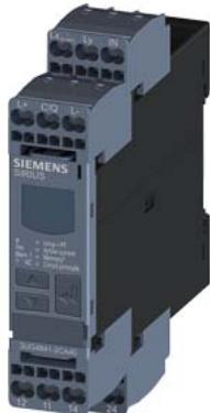
Digital monitoring relay cos phi and current monitoring for IO-Link 90...690 V AC, 0.2...10 A Overshoot and undershoot ON-delay time Tripping delay time Hysteresis 0.1 to 3.0 A 2 change-over contacts, spring-type connection system
