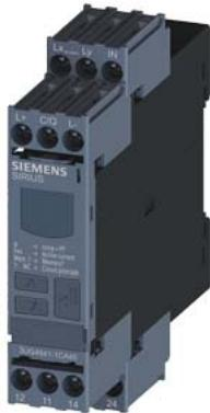
Digital monitoring relay cos phi and current monitoring for IO-Link 90...690 V AC, 0.2...10 A Overshoot and undershoot ON-delay time Tripping delay time Hysteresis 0.1 to 3.0 A 2 change-over contacts, screw terminal
