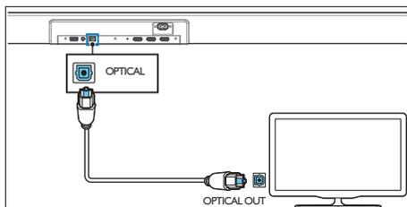
Using an optical cable, connect the **OPTICAL** connector on your Soundbar to the **OPTICAL OUT** connector on the TV or other device.
