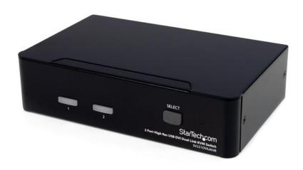
The SV231DVIUAHR 2-Port High Resolution Dual-Link DVI USB KVM Switch provides simple, yet comprehensive control of 2 directly-connected computers, as well as audio switching capability and support for high resolution applications (supports resolutions beyond 1080p: 2560x1600 @ 60Hz, up to 3840 x 2400 at lower refresh rates), offering a superior KVM switching solution that integrates perfectly into demanding imaging, medical, and multimedia environments.
