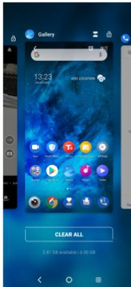
Touch one thumbnail and slide it up to close the application, slide it right/left to switch the applications.
