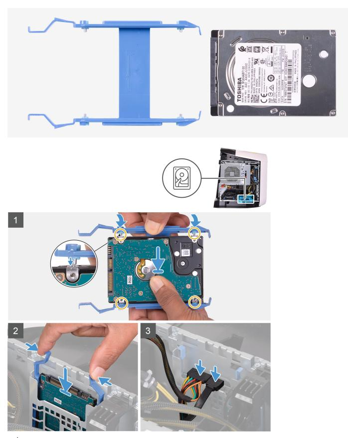
i NOTE: Note the orientation on the hard-drive carrier to replace it correctly.
