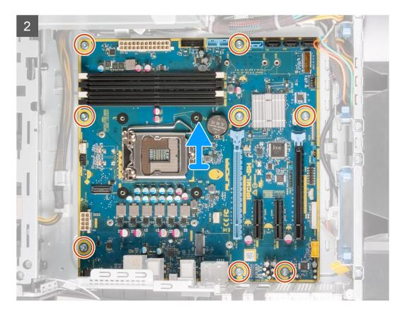
1. Disconnect all the cables connected to the system board.
