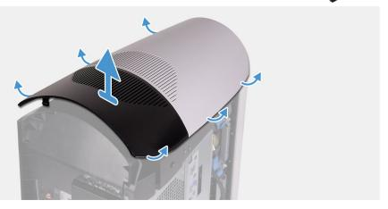
Starting from the rear, pull up on the top cover to release it from the chassis.
