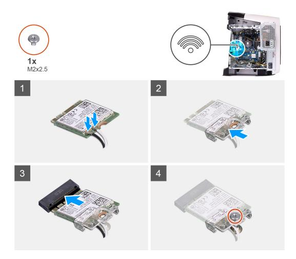
1. Connect the antenna cables to the wireless card.
