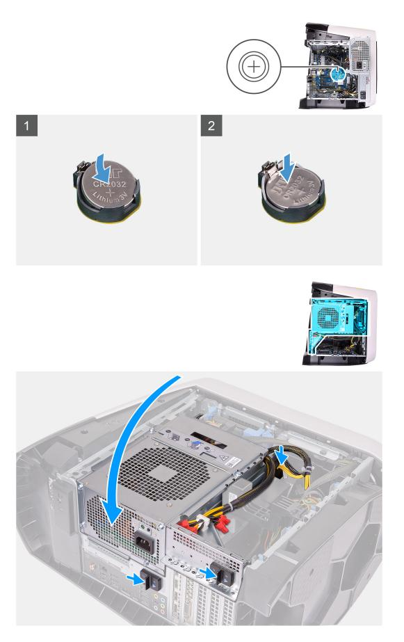
1. Insert a new coin-cell battery (CR2032) into the battery socket with the positive side facing up, and snap the battery into place.
