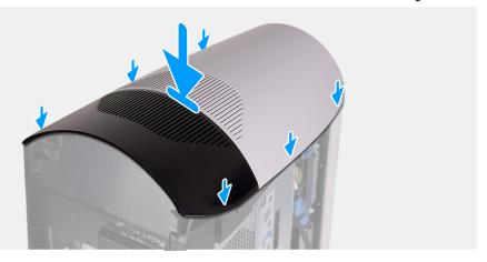
Align the tabs on the top cover with the slots on the chassis and snap the top cover into place.
