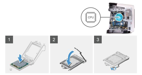
1. Ensure that the release lever on the processor socket is fully extended and the processor cover is fully open.
