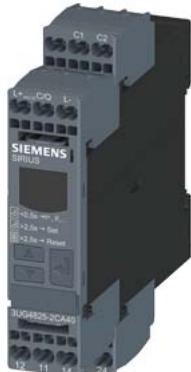
Digital monitoring relay for residual current monitoring with residual-current transformer 3UL23 for IO-Link Setting range 0.03 A to 40 A separate for warning threshold and switch-off value ON delay and tripping delay 0 to 999.9 s Shutdown hysteresis up to 50% Warning hysteresis 5% fixed Width 22.5mm, 2 change-over contacts with or without fault buffer spring-type connection system
