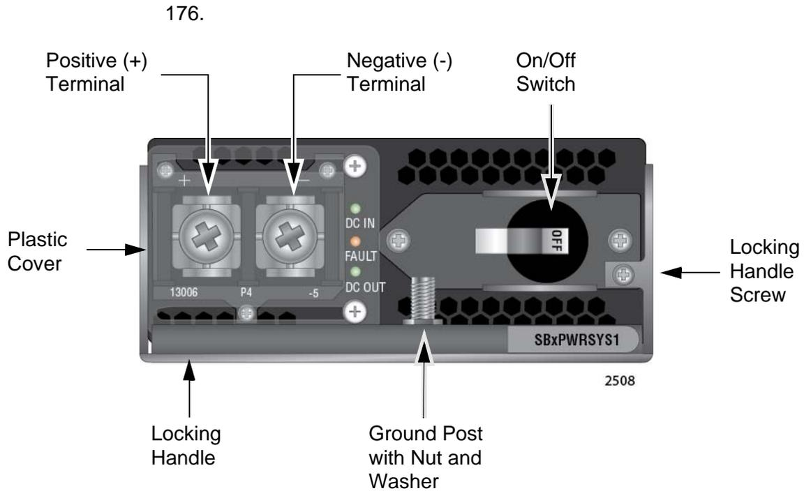
Figure 110. Components of the AT-SBxPWRSYS1 DC Power Supply
