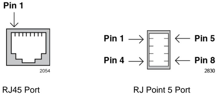
Figure 168. Pin Numbers for the RJ-45 and Point 5 Ports (Front View)
