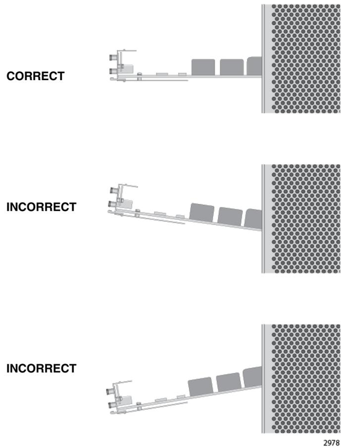
Figure 64. Aligning a Card in a Slot
