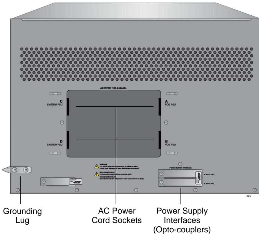
Figure 3. Rear View of the AT-SBx3112 Chassis
