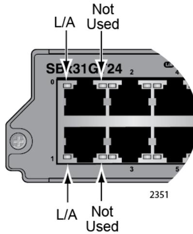
Figure 12. Port LEDs on the AT-SBx31GT24 Line Card
