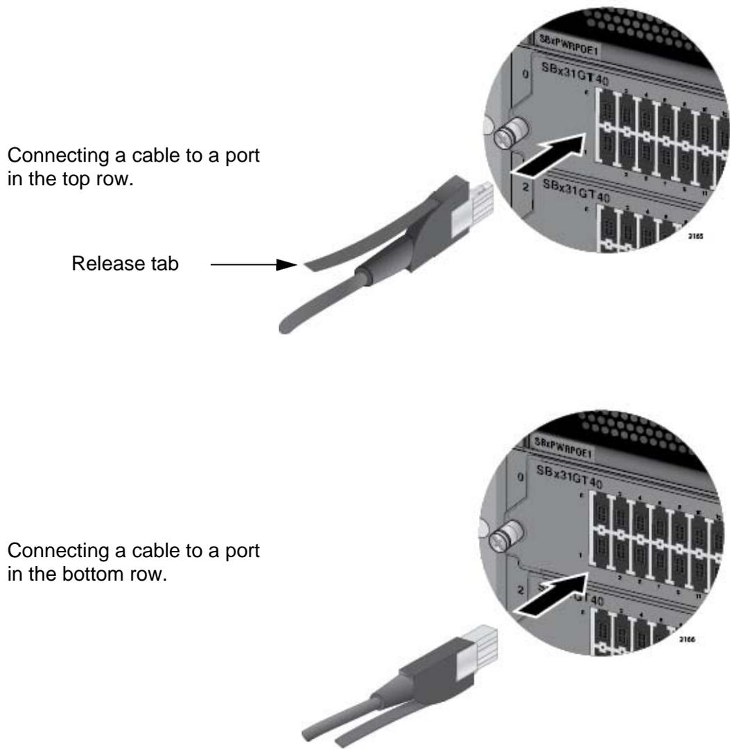
Figure 81. Connecting Cables to Ports on the AT-SBx31GT40 Line Card
