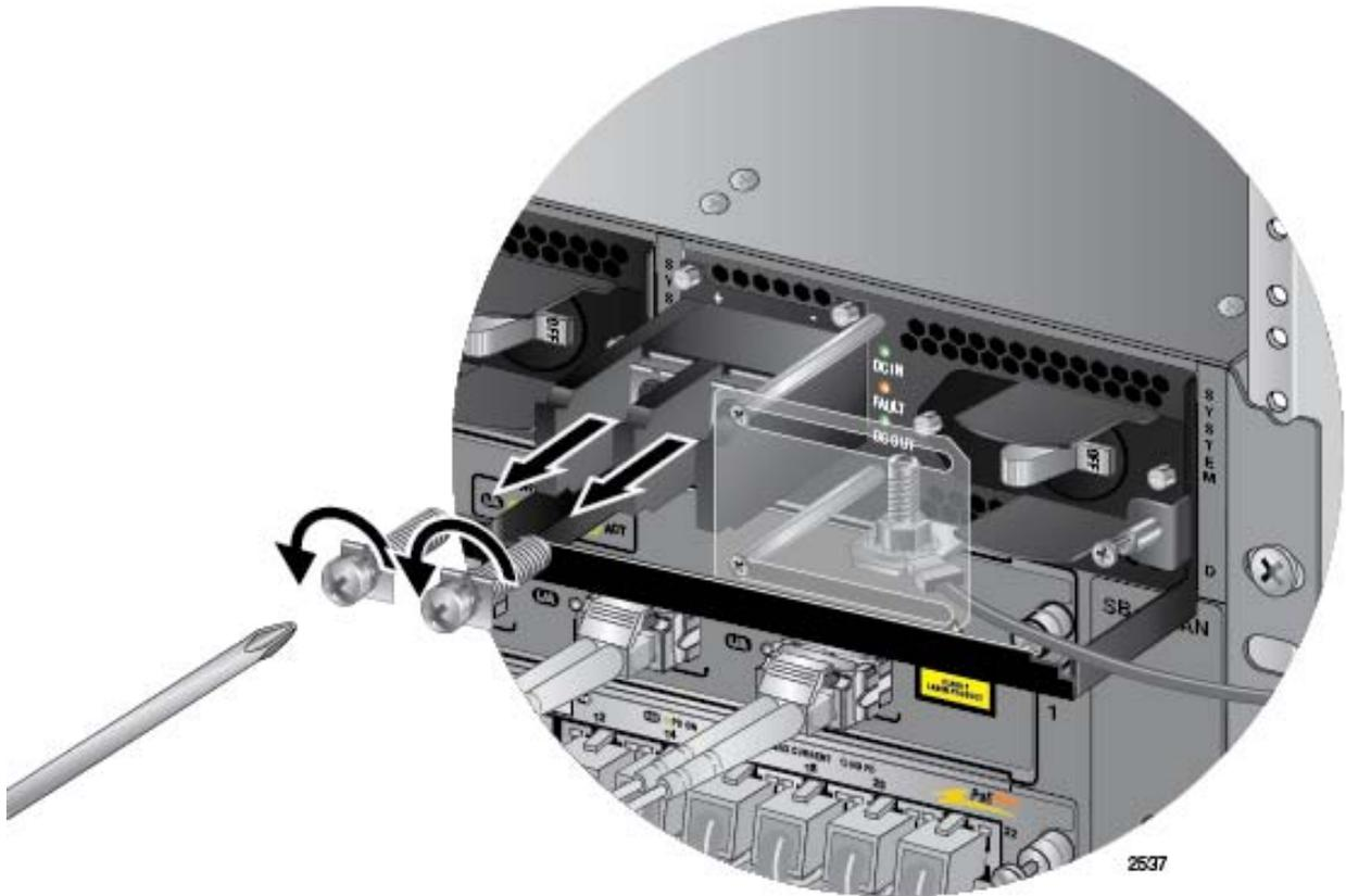
Figure 124. Removing the Terminal Screws
