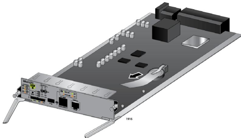
Figure 69. Removing the Battery Insulator
