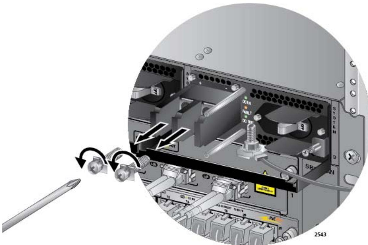
Figure 132. Removing the Terminal Screws
