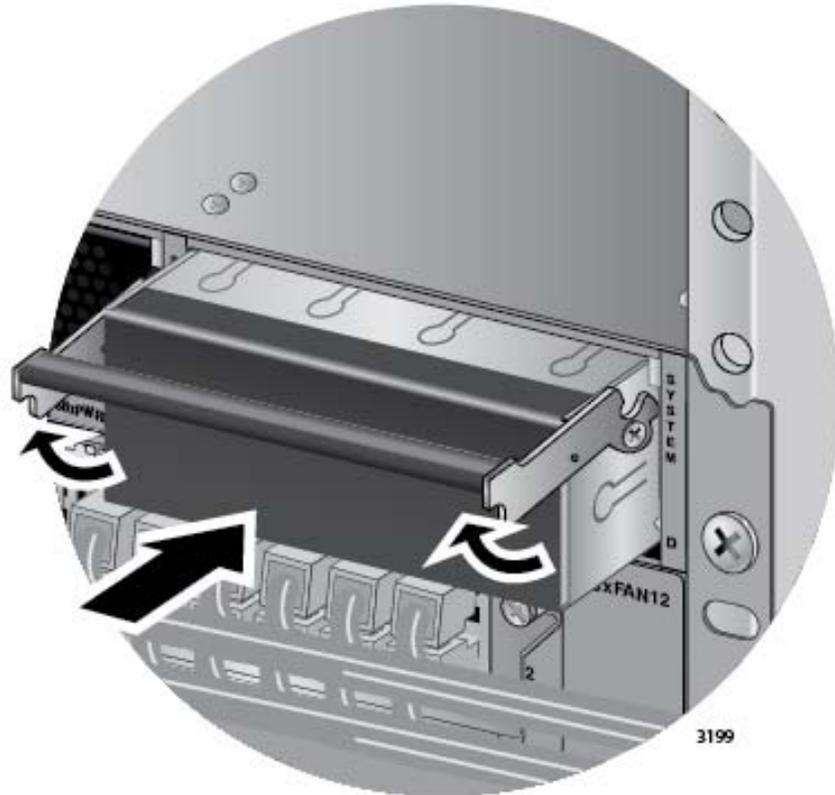
Figure 148. Installing a Blank Power Supply Slot Cover
