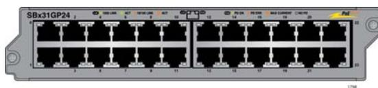
AT-SBx31GP24 Ethernet Line Card with 24 10/100/1000Base-T twisted pair ports, with PoE+.
