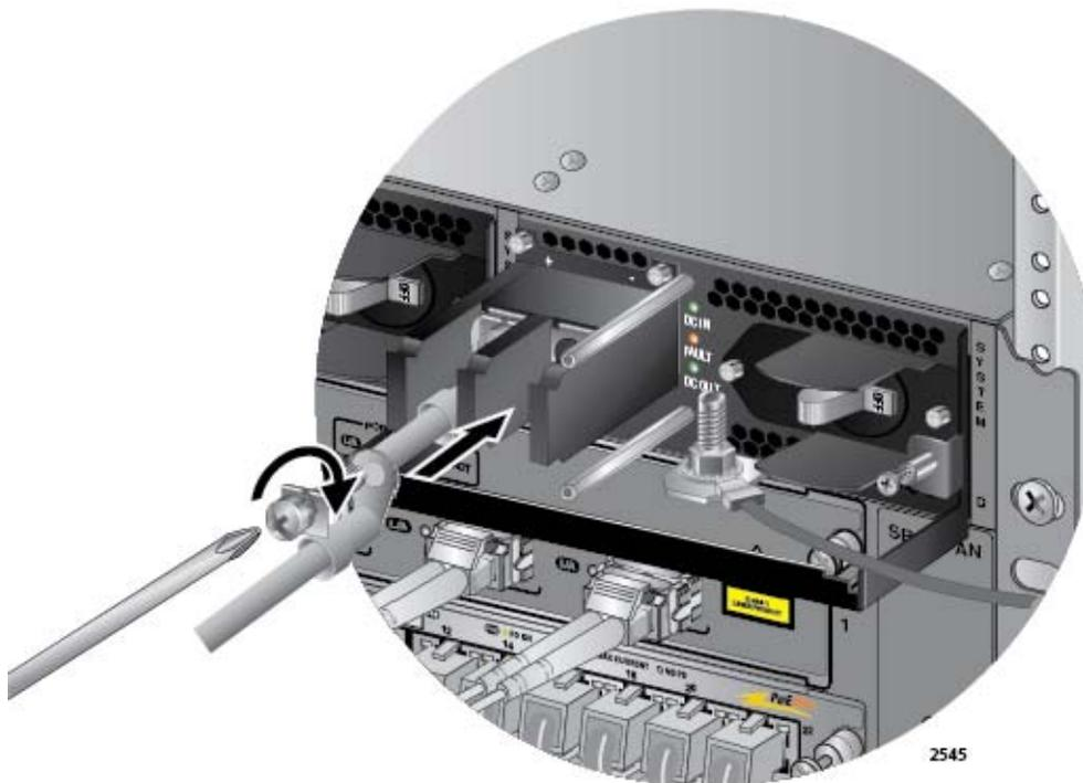
Figure 134. Connecting the Negative (-) Power Wire with a Right Angle Terminal
