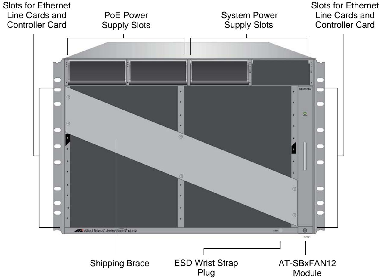
Figure 2. Front View of the AT-SBx3112 Chassis
